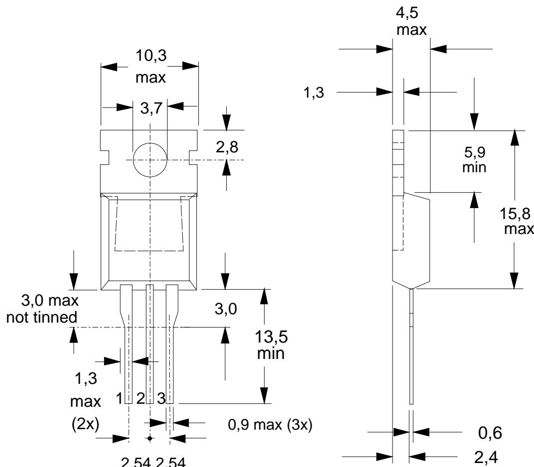
Fig.22. TO220AB; pin 2 connected to mounting base.
