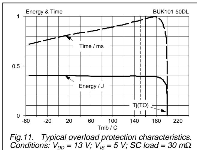
Fig.11. Typical overload protection characteristics.
