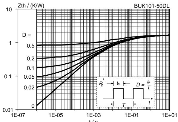
Fig.5. Transient thermal impedance.
