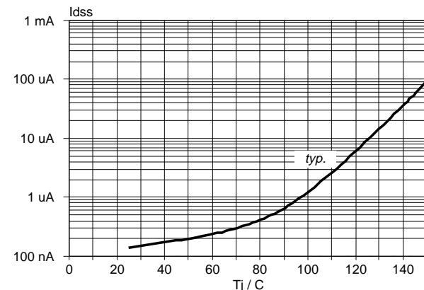
Fig.20. Typical off-state leakage current.
