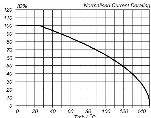
Fig.3. Normalised continuous drain current.
