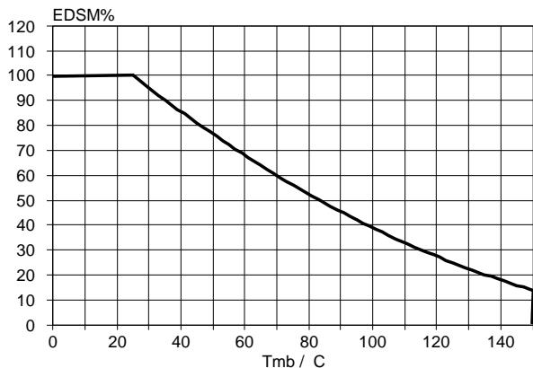
Fig.18. Normalised clamping energy rating.
