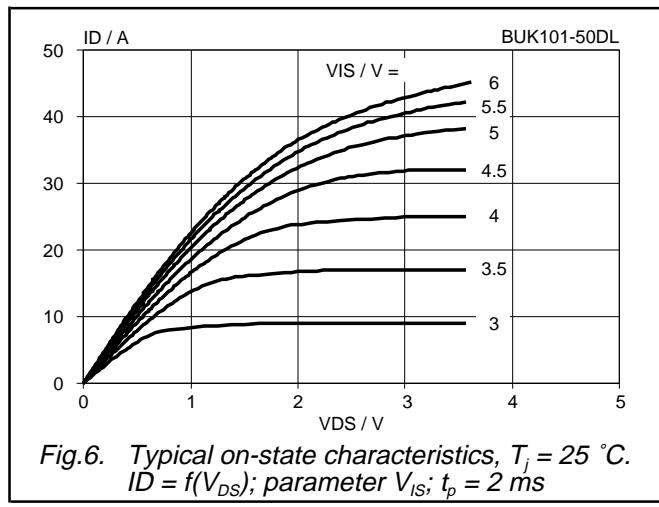
Fig.6. Typical on-state characteristics,  $T_j = 25^\circ\text{C}$ .
