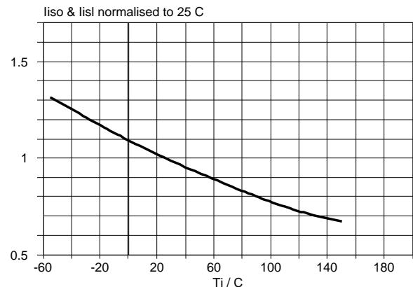
Fig.21. Normalised input currents (normal & latched).
