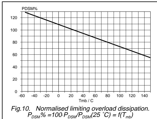
Fig.10. Normalised limiting overload dissipation.
