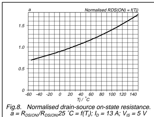
Fig.8. Normalised drain-source on-state resistance.
