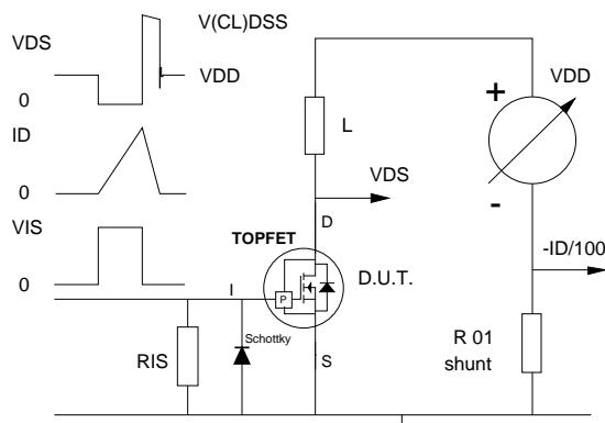
Fig.19. Clamping energy test circuit,  $R_{IS} = 50 \Omega$ .
