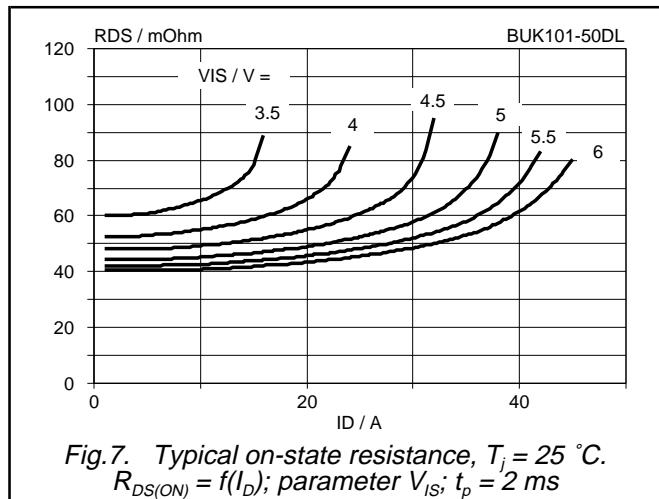
Fig.7. Typical on-state resistance,  $T_j = 25^\circ\text{C}$ .
