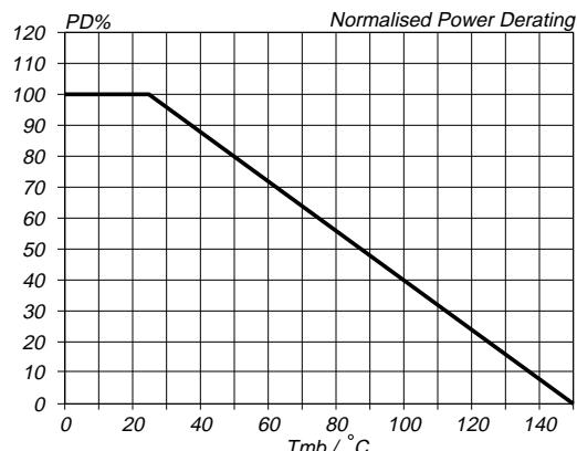
Fig.2. Normalised power dissipation.
