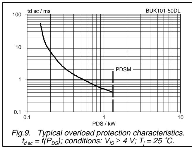
Fig.9. Typical overload protection characteristics.
