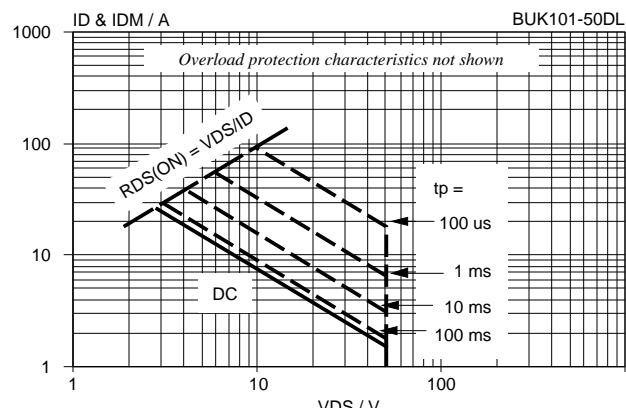
Fig.4. Safe operating area.  $T_{mb} = 25^\circ\text{C}$
