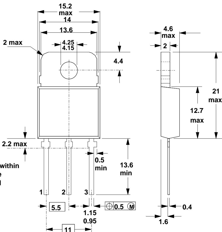
Fig.14. SOT93; pin 2 connected to mounting base.
