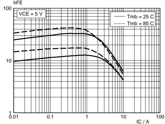
Fig.6. DC current gain.  $h_{FE} = f (I_C)$
