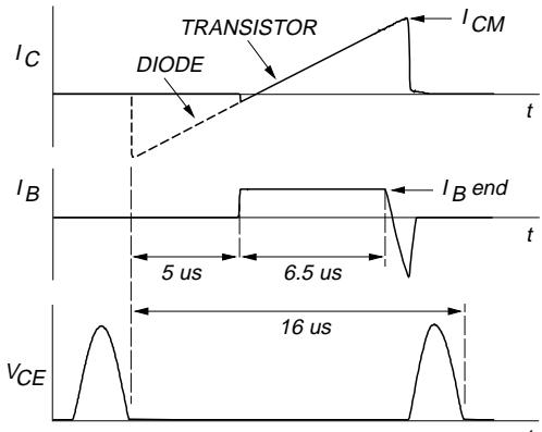
Fig.3. Switching times waveforms (64 kHz).
