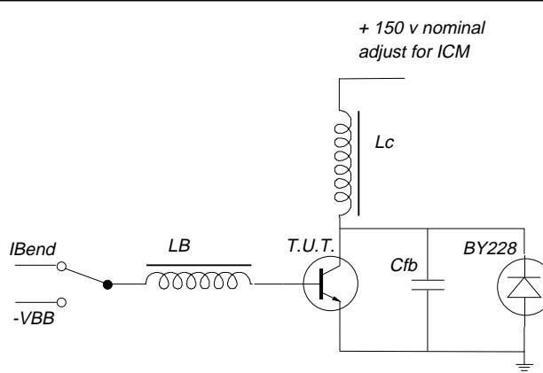
Fig.5. Switching times test circuit.
