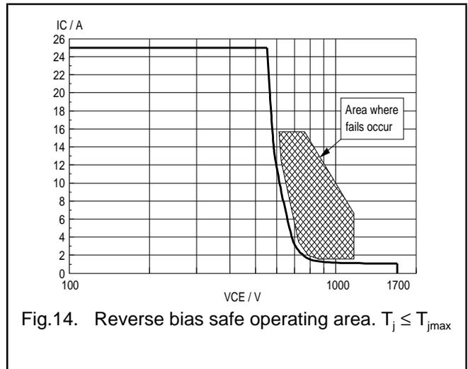
Silicon Diffused Power Transistor
