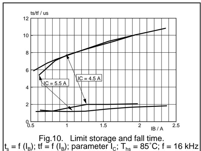
Silicon Diffused Power Transistor
