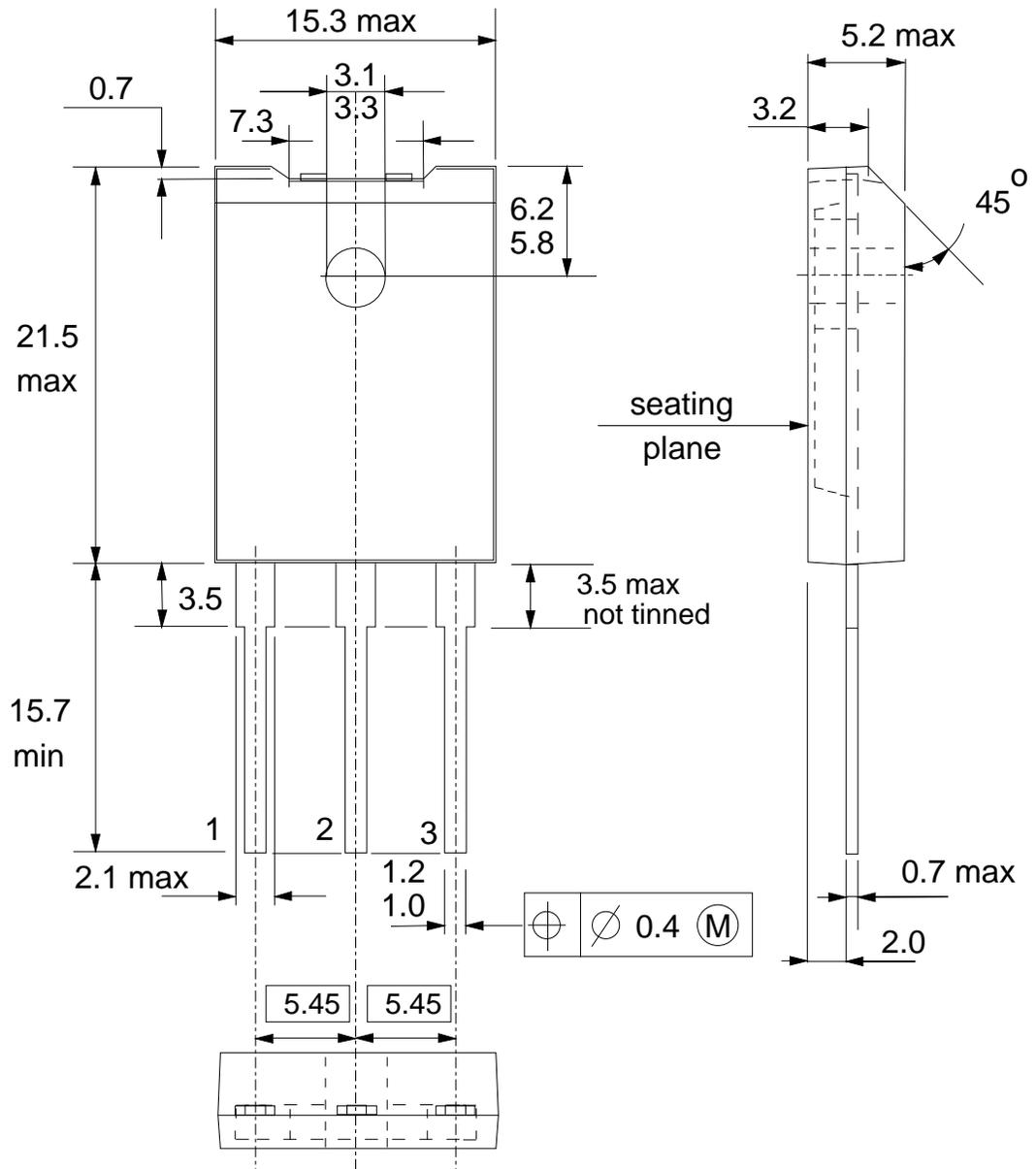
Fig.15. SOT199; The seating plane is electrically isolated from all terminals.
