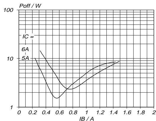
Fig.11. Typical turn-off losses.  $T_j = 85^\circ\text{C}$
