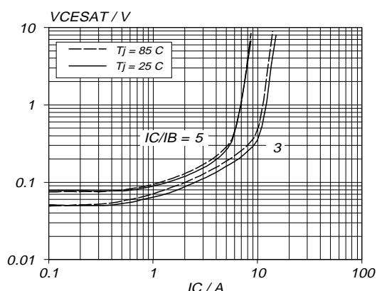
Fig.9. Typical collector-emitter saturation voltage.
