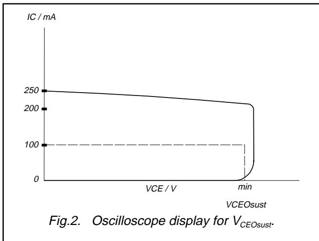
Fig.2. Oscilloscope display for  $V_{CEO}sust$ .
