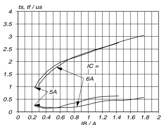
Fig.12. Typical collector storage and fall time.
