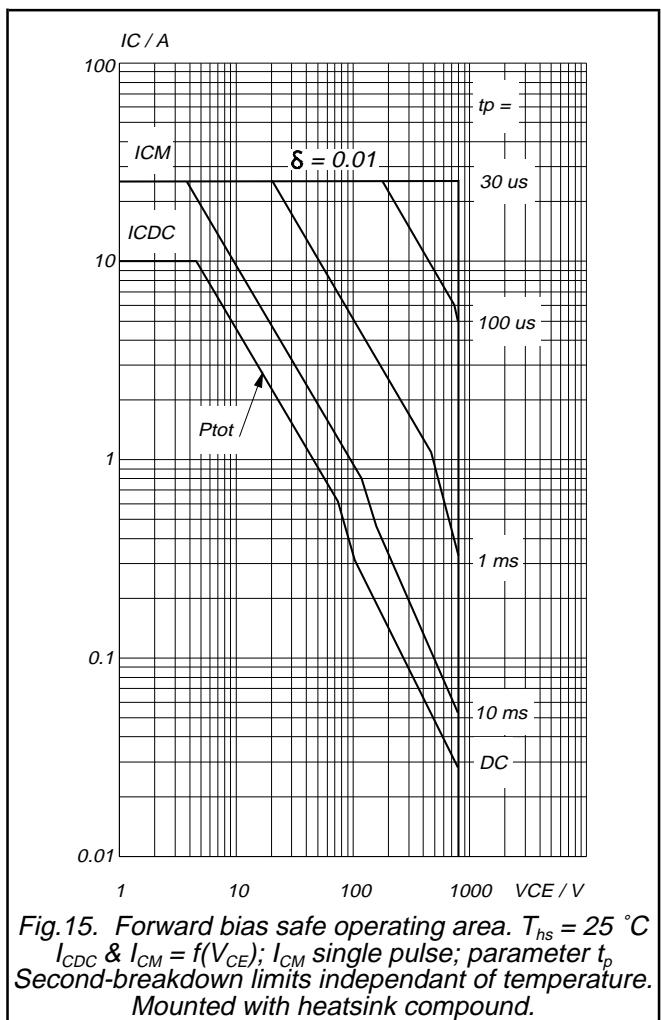
*Fig.15. Forward bias safe operating area.  $T_{hs} = 25^\circ C$*
