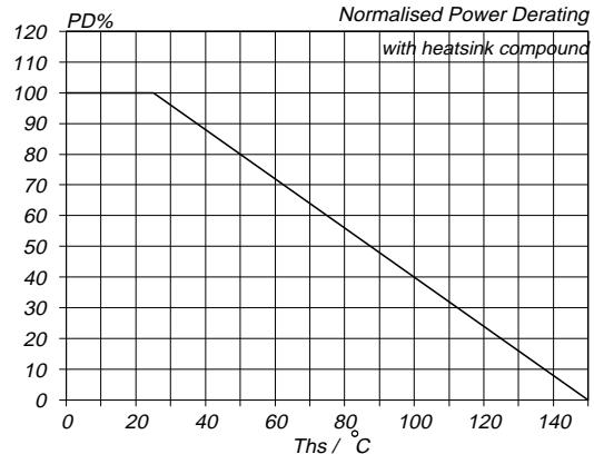
Fig.13. Normalised power dissipation.
