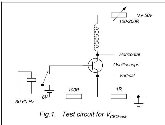
Fig.1. Test circuit for  $V_{CEO}sust$ .
