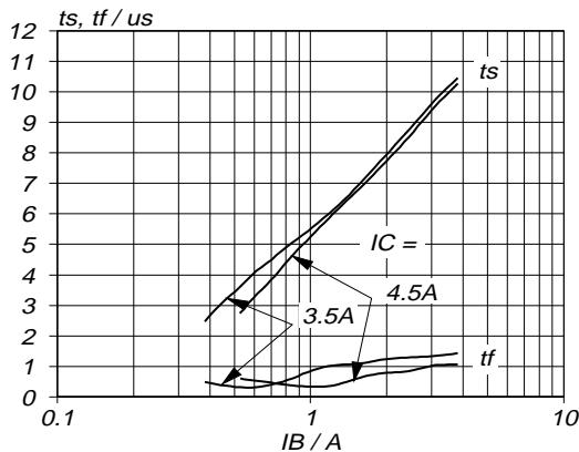
Fig.10. Typical collector storage and fall time.
