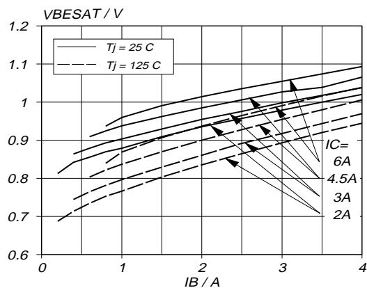
Fig.7. Typical base-emitter saturation voltage.
