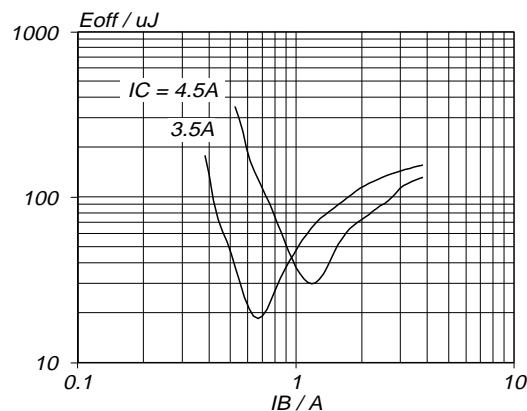
Fig.9. Typical turn-off losses.  $T_j = 85^\circ\text{C}$
