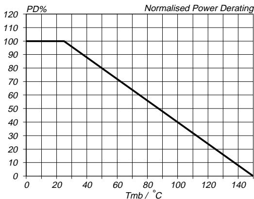
Fig.12. Normalised power dissipation.
