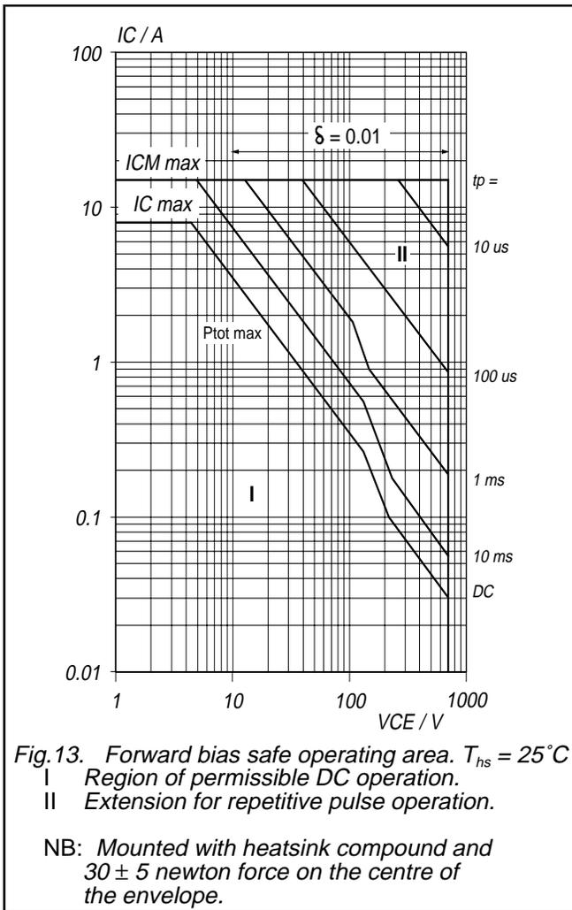
Fig. 13. Forward bias safe operating area.  $T_{hs} = 25^\circ C$
