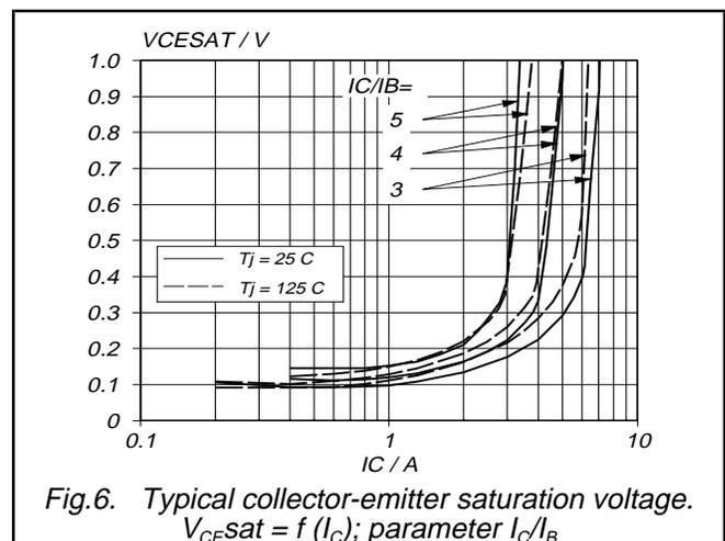
Silicon Diffused Power Transistor
