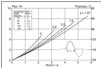
Fig.1. Maximum on-state dissipation,  $P_{tot}$  versus average on-state current,  $I_{T(AV)}$ , where  $a = form \ factor = I_{T(RMS)}/I_{T(AV)}$ .
