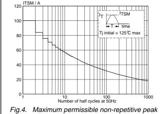
on-state current I<sub>TSM</sub>, versus number of cycles, for sinusoidal currents, f = 50 Hz.
