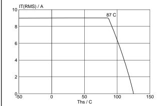
Fig.3. Maximum permissible rms current  $I_{T(RMS)}$ , versus heatsink temperature  $T_{hs}$ .
