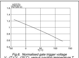
Fig.6. Normalised gate trigger voltage  $V_{GT}(T_j)/V_{GT}(25^{\circ}C)$ , versus junction temperature  $T_{j^{\circ}}$
