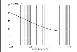
Fig.5. Maximum permissible repetitive rms on-state current  $I_{T(RMS)}$ , versus surge duration, for sinusoidal currents, f = 50 Hz;  $T_{hs} \le 87$ °C.
