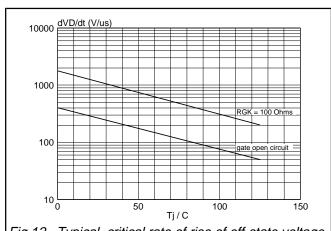
Fig.12. Typical, critical rate of rise of off-state voltage, dV<sub>D</sub>/dt versus junction temperature T<sub>j</sub>.
