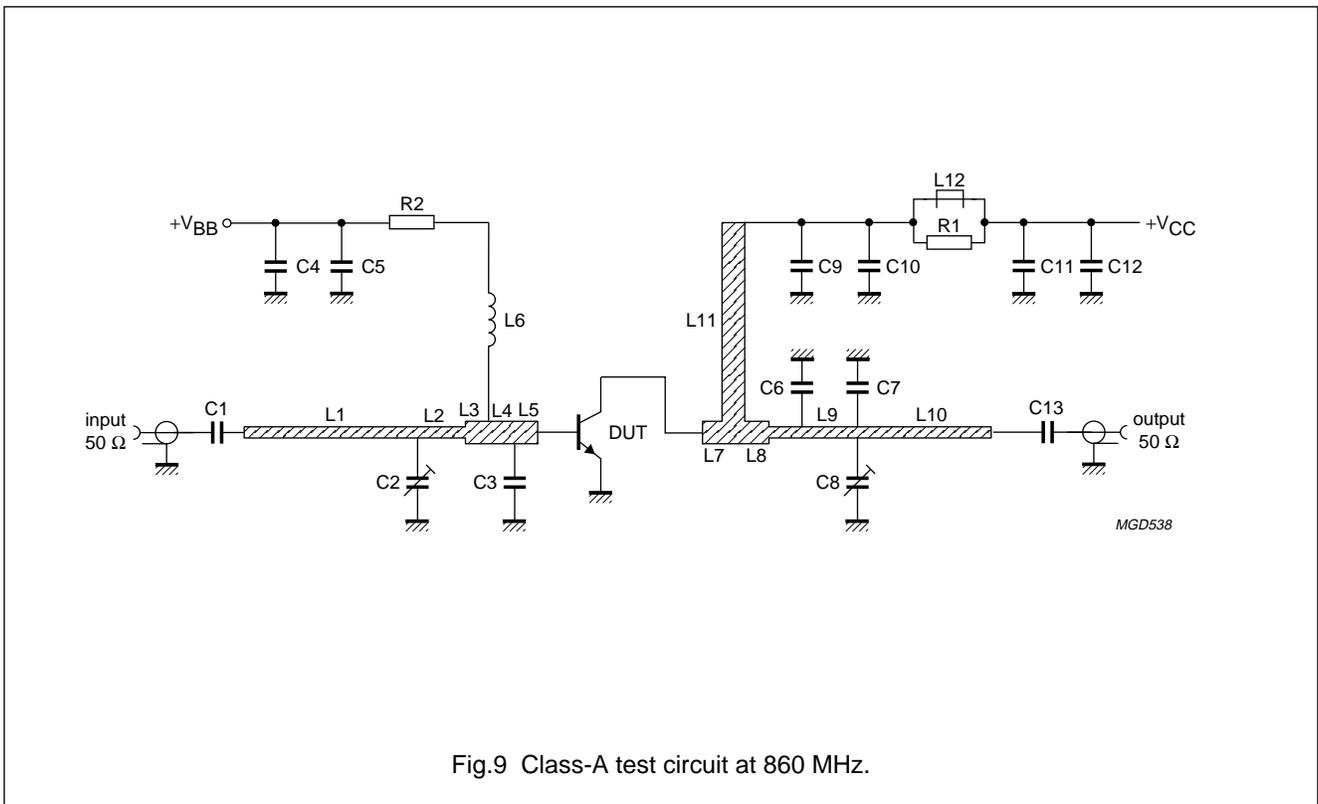
UHF linear power transistor
