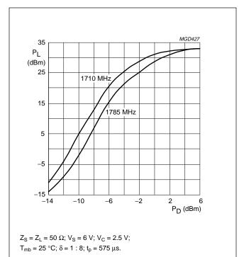
Fig.3 Load power as a function of drive power; typical values.
