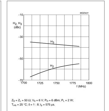
Fig.7 Harmonics as a function of frequency; typical values.
