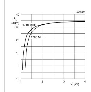
$$\begin{split} Z_S = Z_L = 50~\Omega;~V_S = 6~V;~P_D = 6~dBm;\\ T_{mb} = 25~^{\circ}C;~\delta = 1:8;~t_p = 575~\mu s. \end{split}$$
