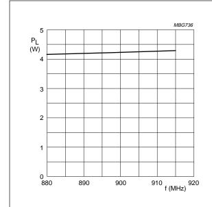
$Z_S = Z_L = 50~\Omega;~P_D = 3~dBm;~V_S = 6~V;$   $V_C = 4~V;~T_{mb} = 25~^{\circ}C;~\delta = 1~:8;~t_p = 575~\mu s.$
