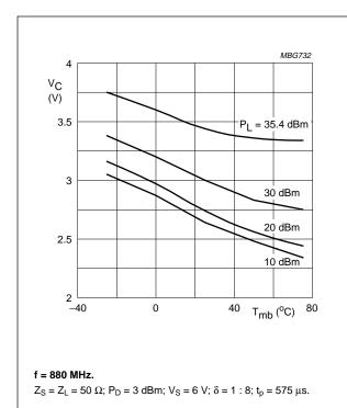
Fig.14 Control voltage as a function of mounting base temperature; typical values.
