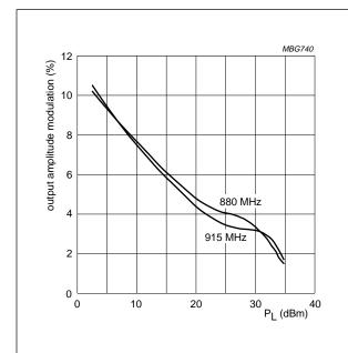
$$\begin{split} Z_S = Z_L = 50~\Omega;~P_D = 3~dBm;~V_S = 6~V;~T_{mb} = 25~^{\circ}C;\\ \delta = 1:8;~t_p = 575~\mu s;~input~amplitude~modulation = 3\%. \end{split}$$
