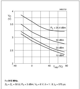
Fig.15 Control voltage as a function of mounting base temperature; typical values.
