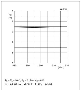
Fig.7 Control voltage as a function of frequency; typical values.
