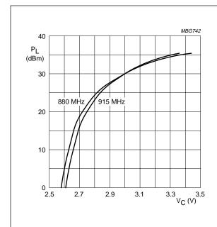
$$\begin{split} Z_S = Z_L = 50~\Omega;~P_D = 3~\text{dBm};~V_S = 6~\text{V};\\ T_{mb} = 25~^{\circ}\text{C};~\delta = 1~:~8;~t_p = 575~\mu\text{s}. \end{split}$$
