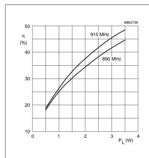
$$\begin{split} Z_S = Z_L = 50 \ \Omega; \ P_D = 3 \ dBm; \ V_S = 6 \ V; \\ T_{mb} = 25 \ ^{\circ}C; \ \delta = 1 : 8; \ t_p = 575 \ \mu s. \end{split}$$
