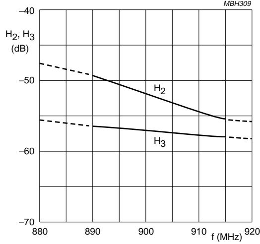
$Z_S = Z_L = 50 \Omega$ ;  $P_D = 1 \text{ mW}$ ;  $V_{S1} = V_{S2} = V_{S3} = 7.2 \text{ V}$ ;  $P_L = 1.7 \text{ W}$ ;
