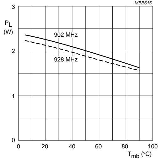
$Z_S = Z_L = 50 \Omega$ ;  $P_D = 1 \text{ mW}$ ;  $V_{S1} = V_{S2} = V_{S3} = 7.2 \text{ V}$ ;  $V_C = 4.5 \text{ V}$ .
