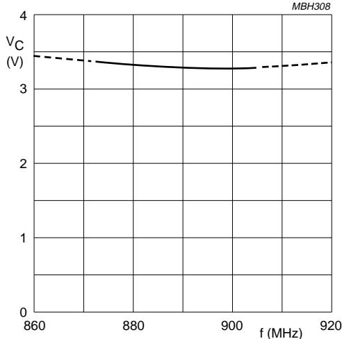
$Z_S = Z_L = 50 \Omega$ ;  $P_D = 1 \text{ mW}$ ;  $V_{S1} = V_{S2} = V_{S3} = 7.2 \text{ V}$ ;  $P_L = 1.7 \text{ W}$ ;
