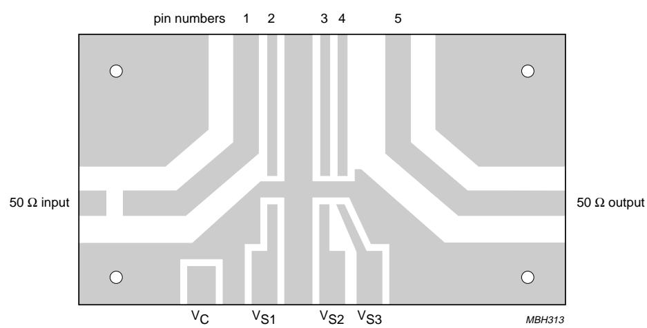
Fig.36 Printed circuit board test-fixture.
