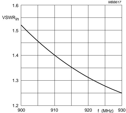
$Z_S = Z_L = 50 \Omega$ ;  $P_D = 1 \text{ mW}$ ;  $V_{S1} = V_{S2} = V_{S3} = 7.2 \text{ V}$ ;  $P_L = 1.7 \text{ W}$ ;
