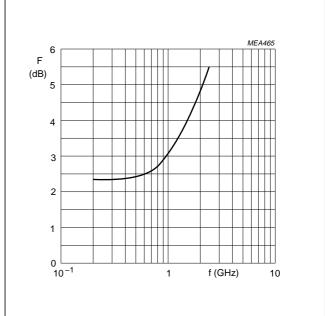
$I_c$  = -2 mA;  $V_{CE}$  = -10 V;  $Z_s$  = opt.;  $T_{amb}$  = 25 °C.
