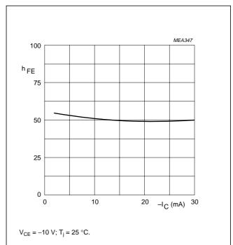
Fig.3 DC current gain as a function of collector current.
