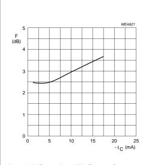
$V_{CE} = -10 \text{ V}; \ \ Z_s = opt.; \, f = 500 \text{ MHz}; \, T_{amb} = 25 \,\,^{\circ}\text{C}.$
