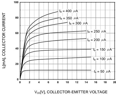
Figure 1. Static Characteristic
