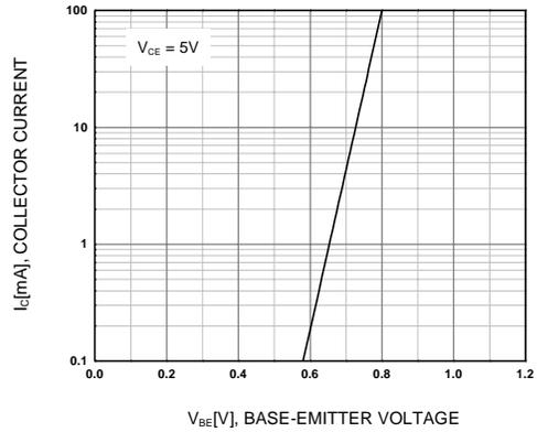
Figure 2. Transfer Characteristic
