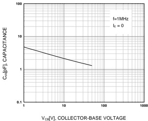
Figure 5. Output Capacitance
