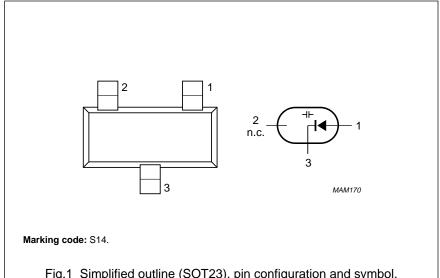
Fig.1 Simplified outline (SOT23), pin configuration and symbol.
