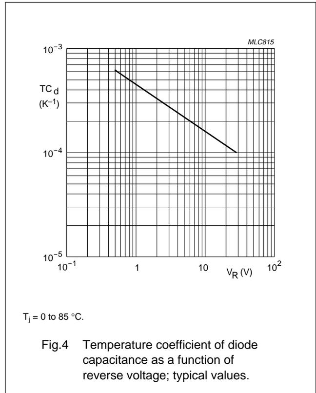
UHF variable capacitance diode
