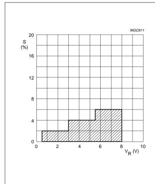
Fig.5 Capacitance matching as a function of reverse voltage; typical values.
