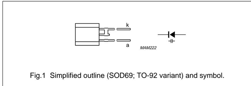
Fig.1 Simplified outline (SOD69; TO-92 variant) and symbol.
