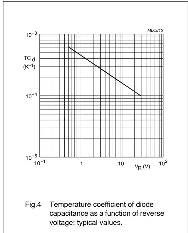
AM variable capacitance diode
