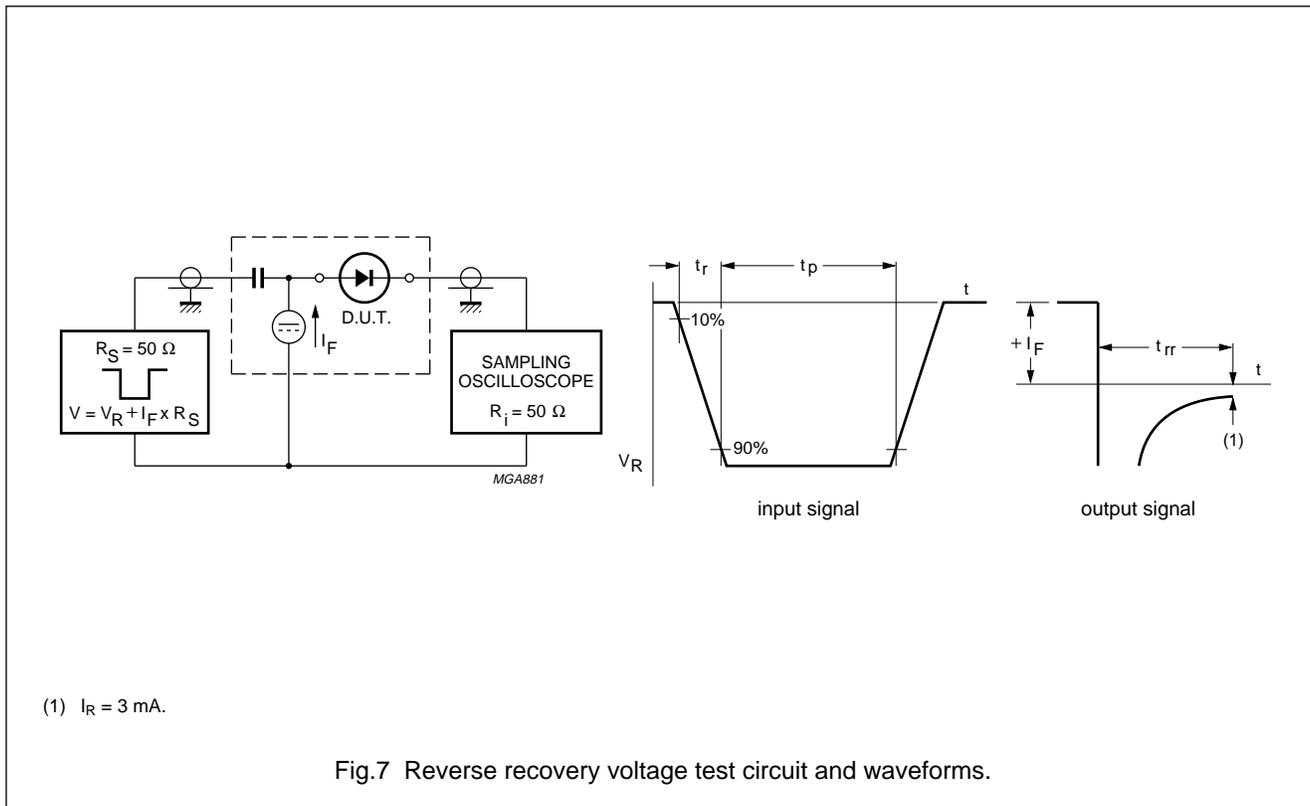
Fig.7 Reverse recovery voltage test circuit and waveforms.
