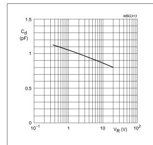
$f = 1 \text{ MHz}; T_j = 25 \,^{\circ}\text{C}.$
