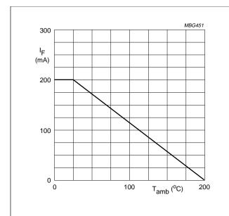
Device mounted on an FR4 printed-circuit board; lead length 10 mm.
