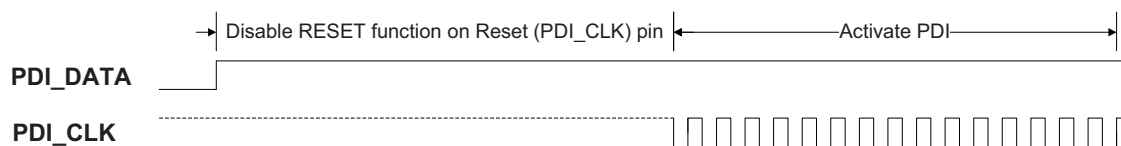
Figure 32-3. PDI physical layer enable sequence.
