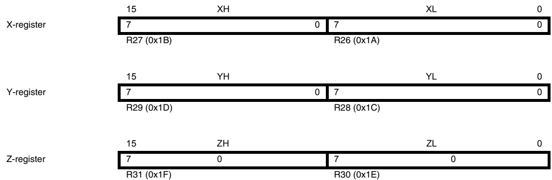
Figure 4-3. The X-, Y-, and Z-registers
