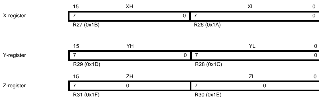
Figure 6-3. The X-, Y-, and Z-registers
