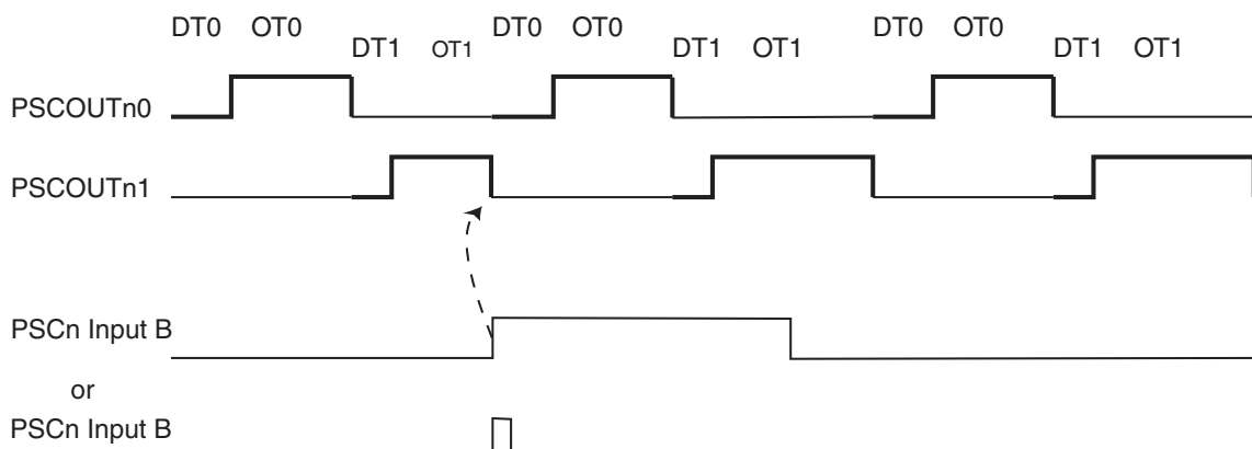
Figure 13-26. PSCR behavior versus PSCr Input B in Mode 8
