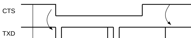
Figure 20-16. Transmitter Behavior when Operating with Hardware Handshaking
