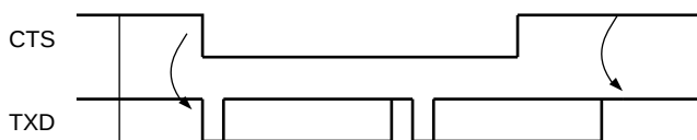
Figure 25-28. Transmitter Behavior when Operating with Hardware Handshaking
