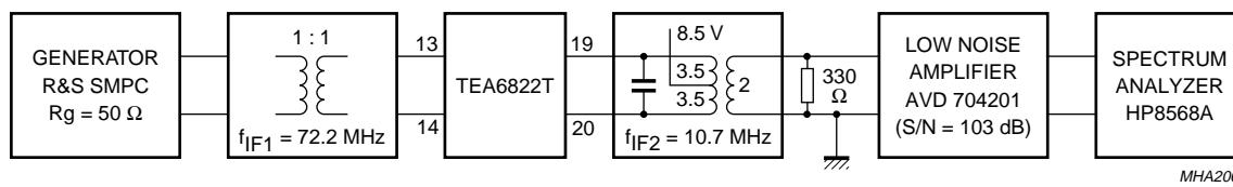
Fig.3 Test circuit FM mixer.
