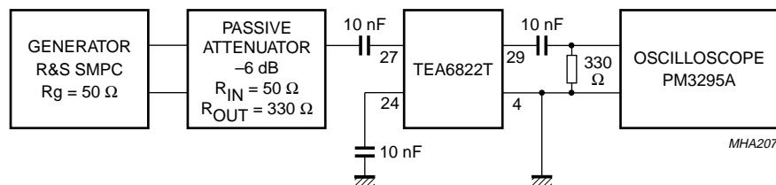
Fig.4 Test circuit IF-amplifier.
