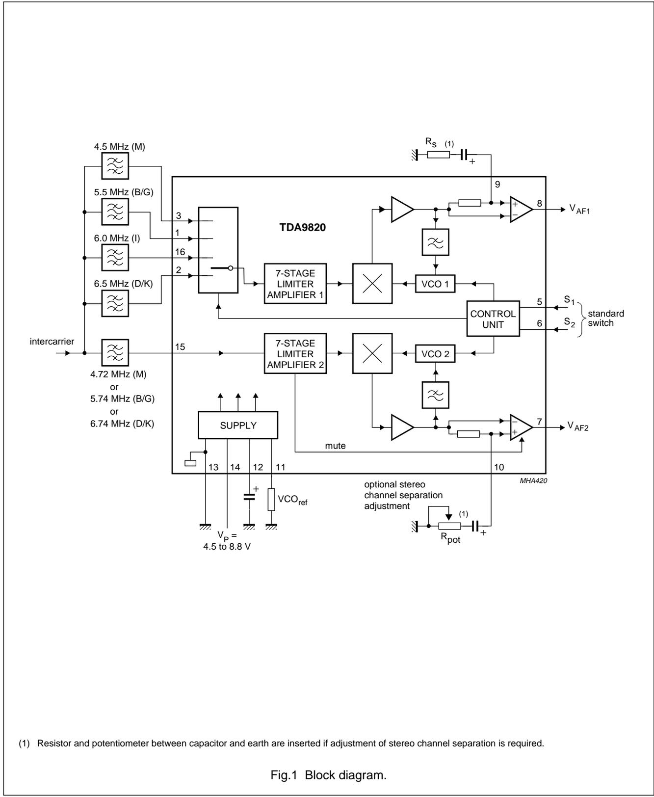
(1) Resistor and potentiometer between capacitor and earth are inserted if adjustment of stereo channel separation is required.
