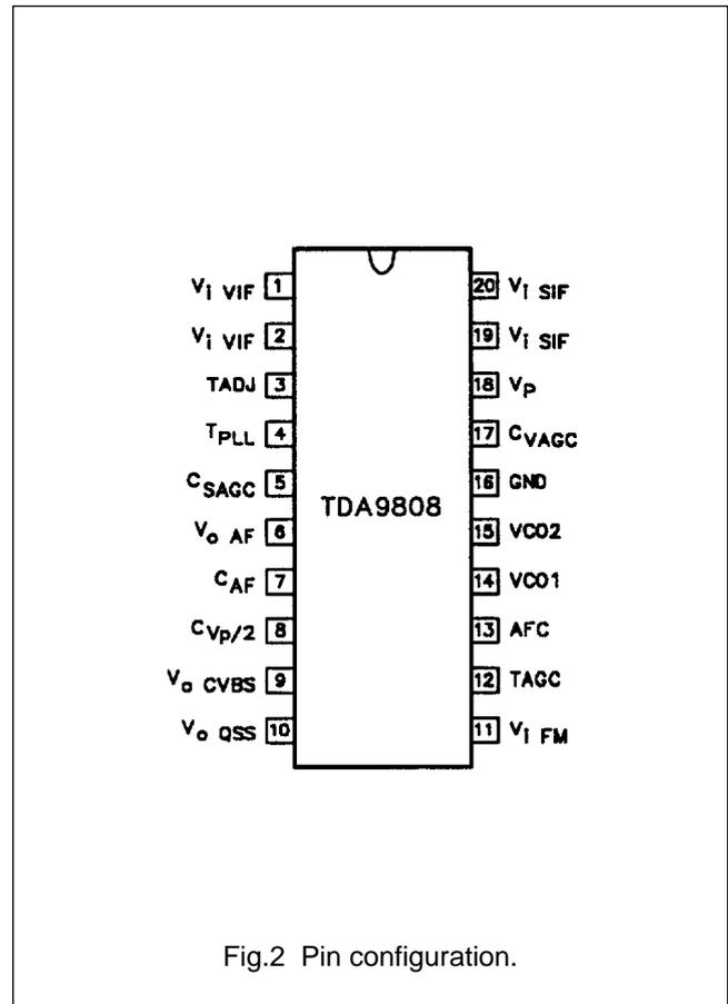
Fig.2 Pin configuration.
