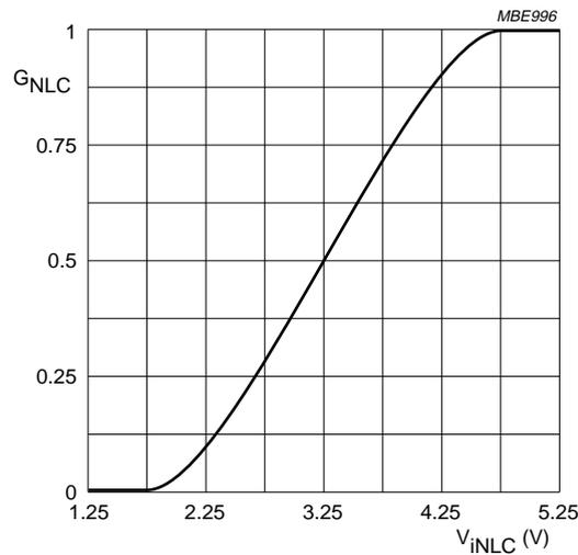
Fig.5 Non-linear amplifier gain as a function of input voltage at pin NLC.
