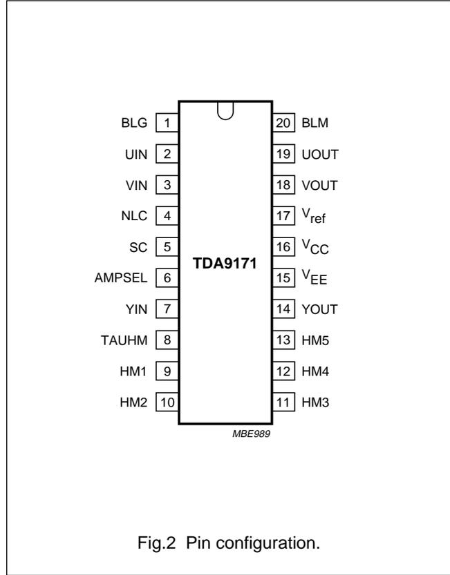
Fig.2 Pin configuration.
