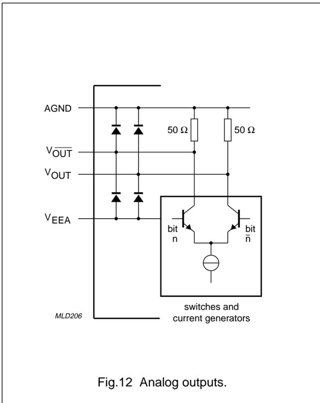
Fig.12 Analog outputs.
