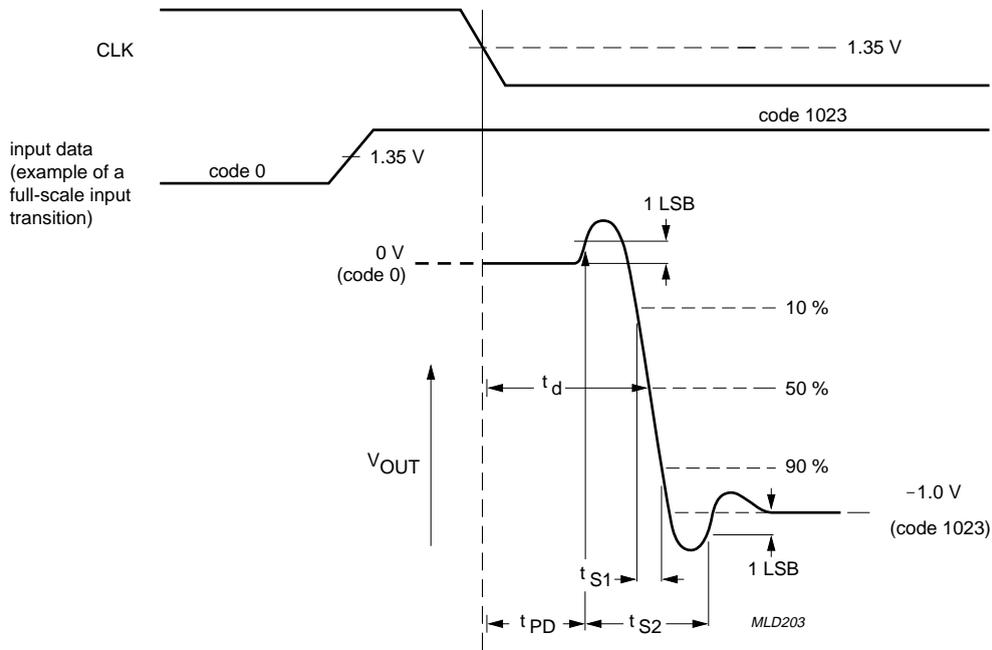
Fig.9 Switching characteristics.
