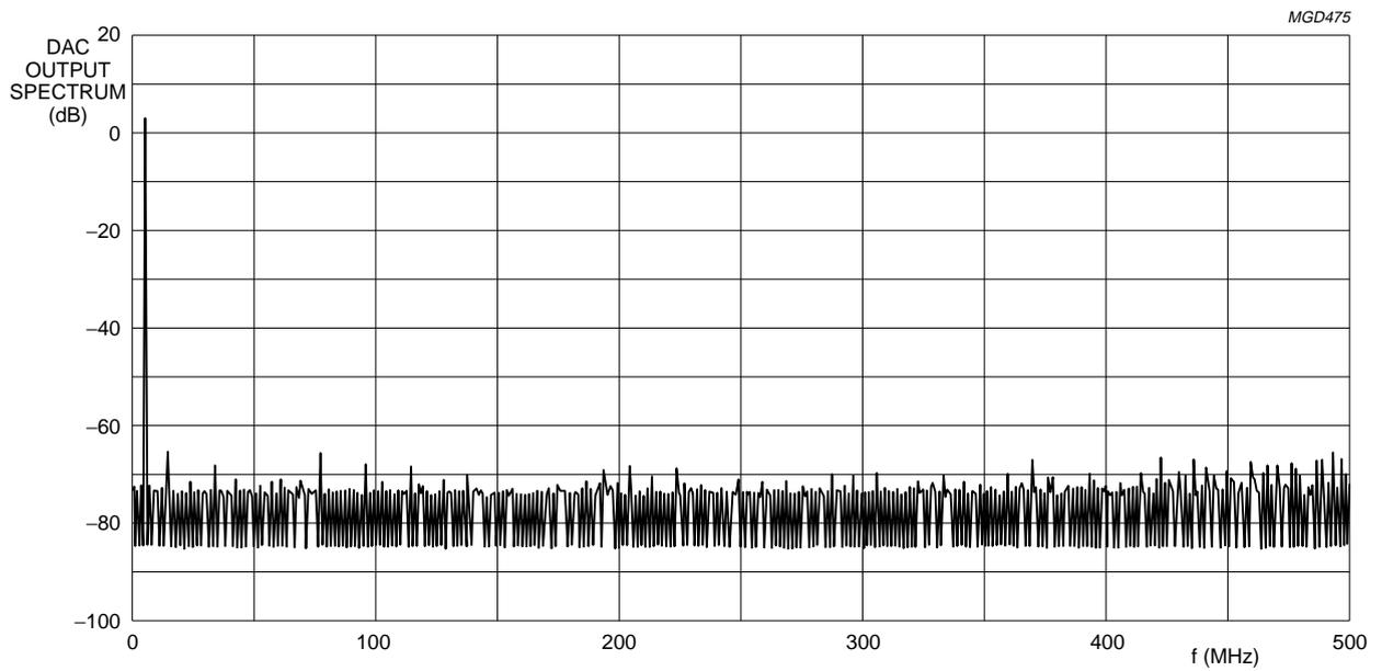
Fig.4 Typical output spectrum;  $f_{clk} = 1000$  MHz;  $f_{OUT} = 10$  MHz.
