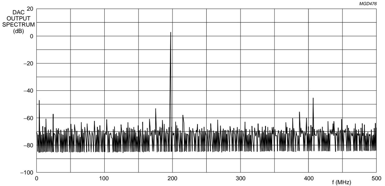
Fig.7 Typical output spectrum;  $f_{clk} = 1000$  MHz;  $f_{OUT} = 200$  MHz.
