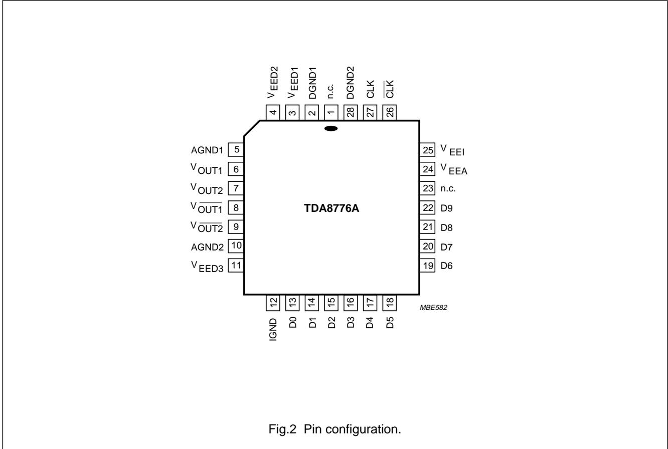
Fig.2 Pin configuration.
