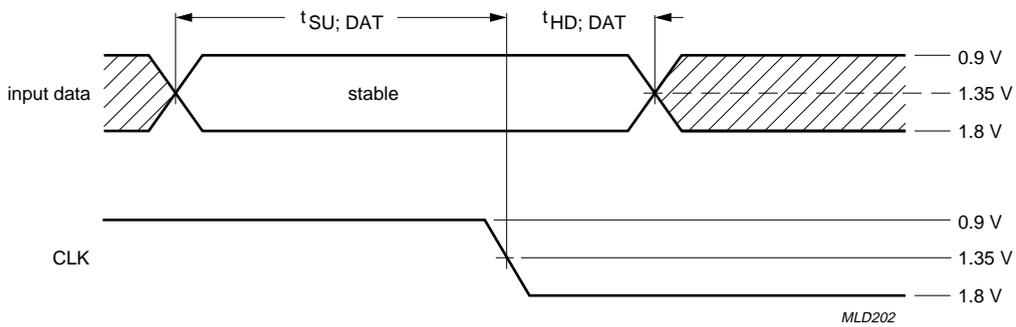
The shaded areas indicate when the input data may change and be correctly registered. Data input update must be completed within  $t_{bf}$  ns after the falling edge of the clock ( $t_{SU; DAT}$  is negative;  $t_{bf}$  ns). Data must be held at least  $t_{bf}$  ns after the falling edge ( $t_{HD; DAT} = t_{bf}$  ns).
