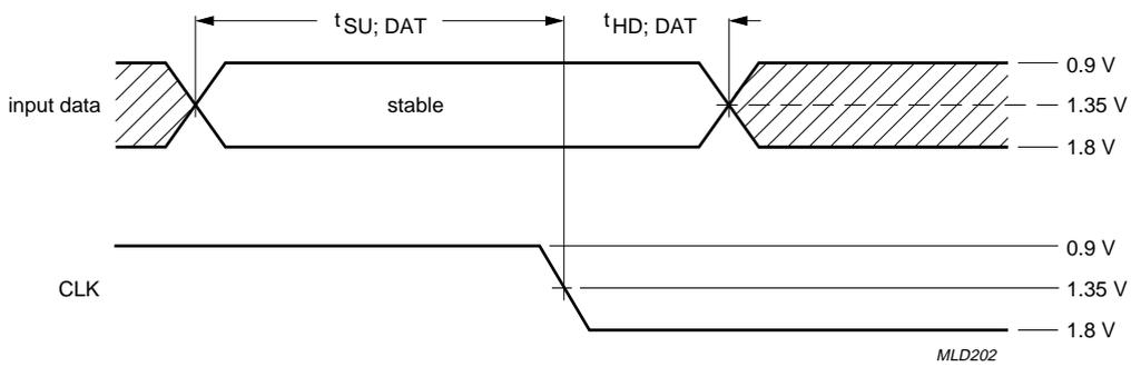
The shaded areas indicate when the input data may change and be correctly registered. Data input update must be completed within  $t_{bf}$  ns after the falling edge of the clock ( $t_{SU; DAT}$  is negative;  $t_{bf}$  ns). Data must be held at least  $t_{bf}$  ns after the falling edge ( $t_{HD; DAT} = t_{bf}$  ns).
