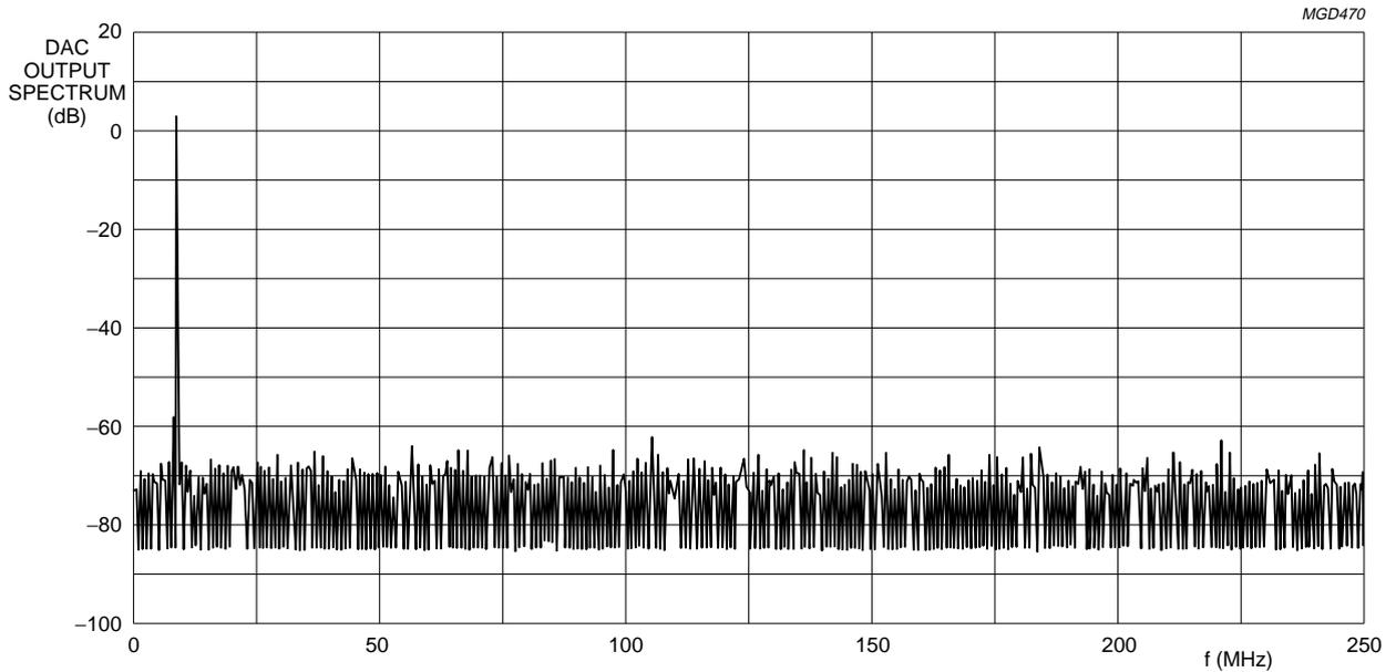
Fig.4 Typical output spectrum;  $f_{clk} = 500$  MHz;  $f_{OUT} = 10$  MHz.
