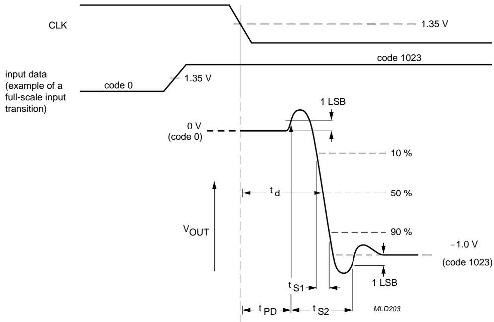
Fig.9 Switching characteristics.
