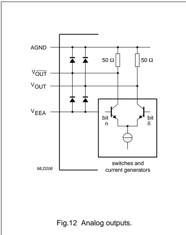
Fig.12 Analog outputs.
