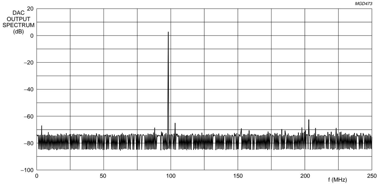
Fig.7 Typical output spectrum;  $f_{clk} = 500$  MHz;  $f_{OUT} = 100$  MHz.
