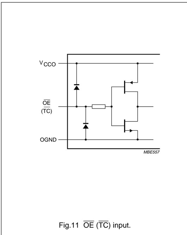
Fig.11  $\overline{OE}$  (TC) input.
