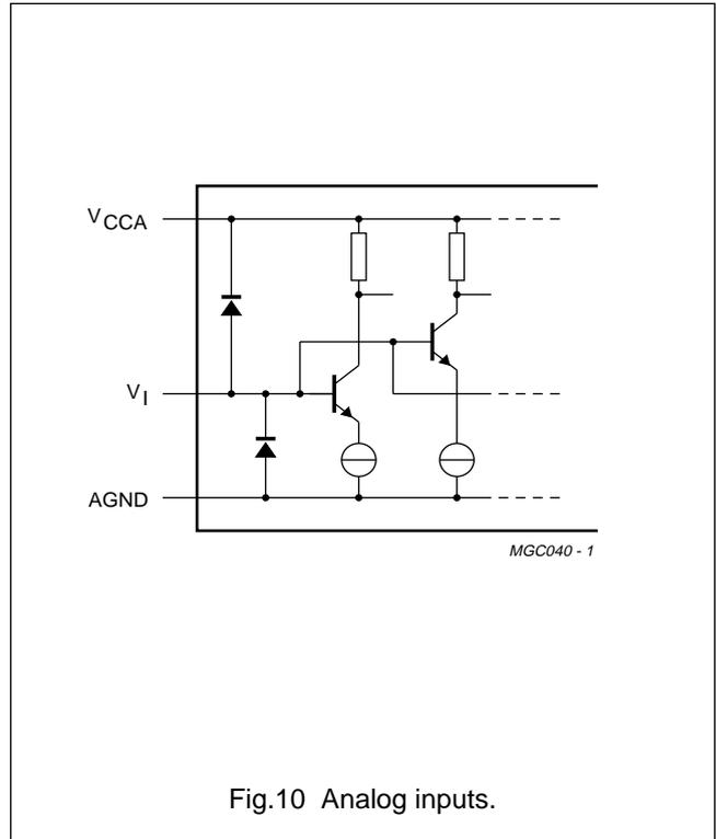
Fig.10 Analog inputs.
