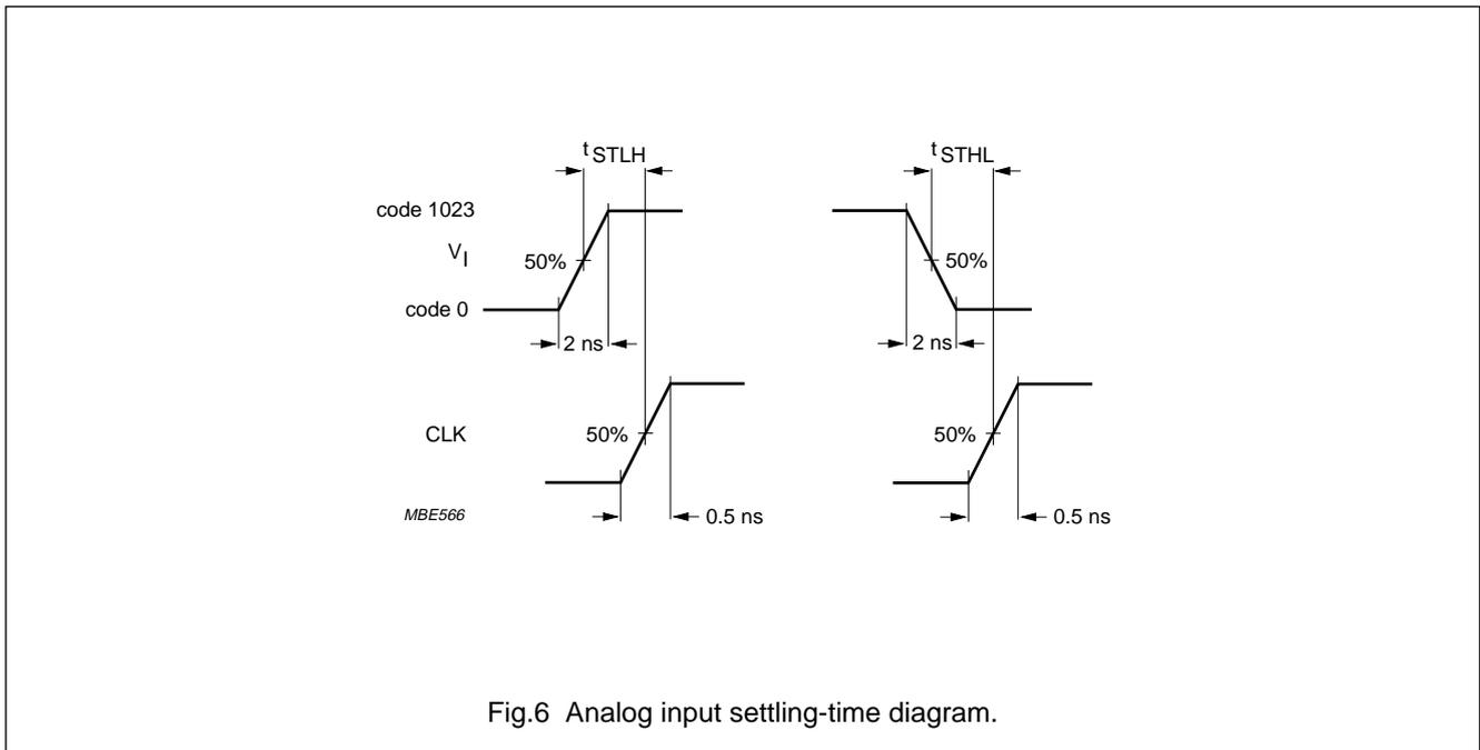
Fig.6 Analog input settling-time diagram.
