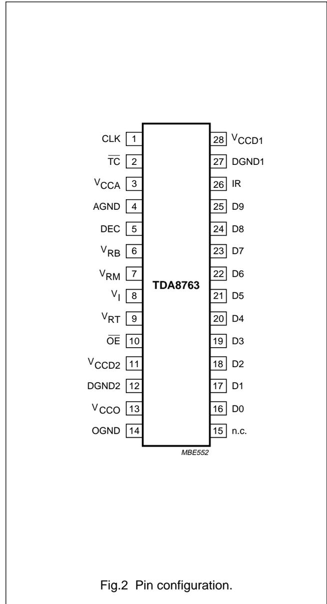
Fig.2 Pin configuration.
