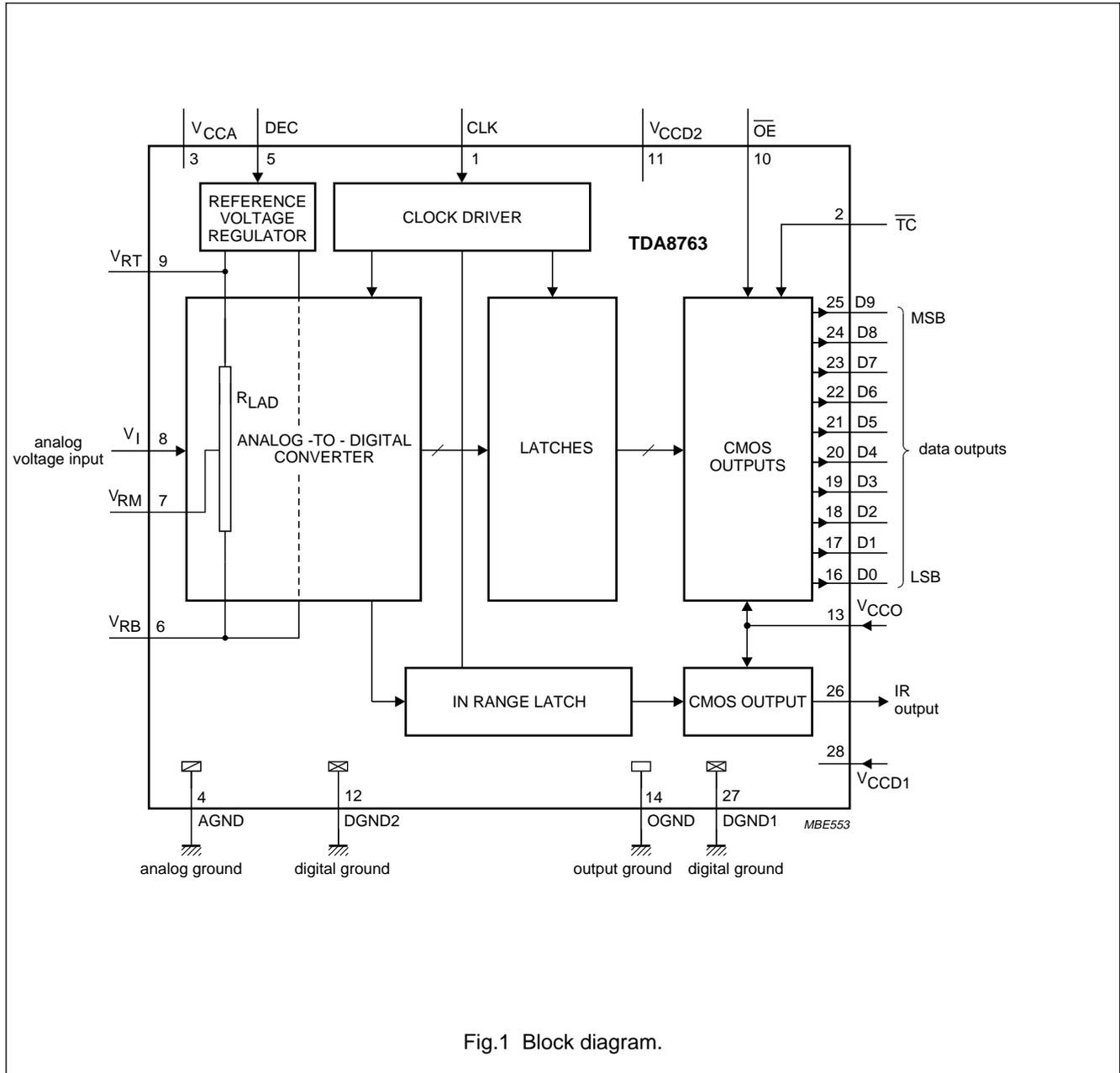
Fig.1 Block diagram.
