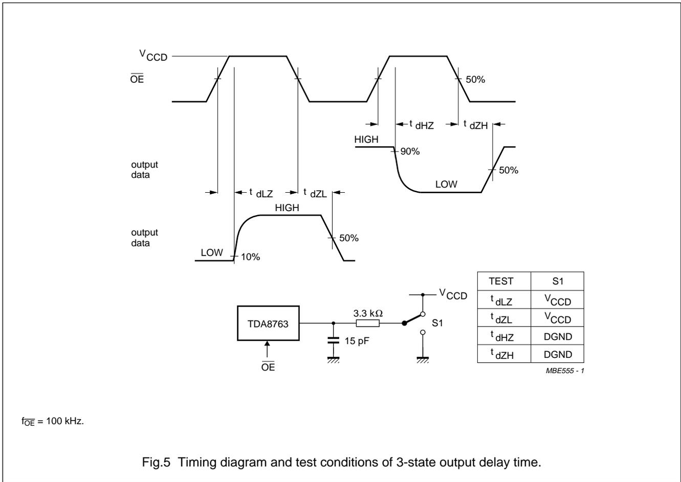
Fig.5 Timing diagram and test conditions of 3-state output delay time.
