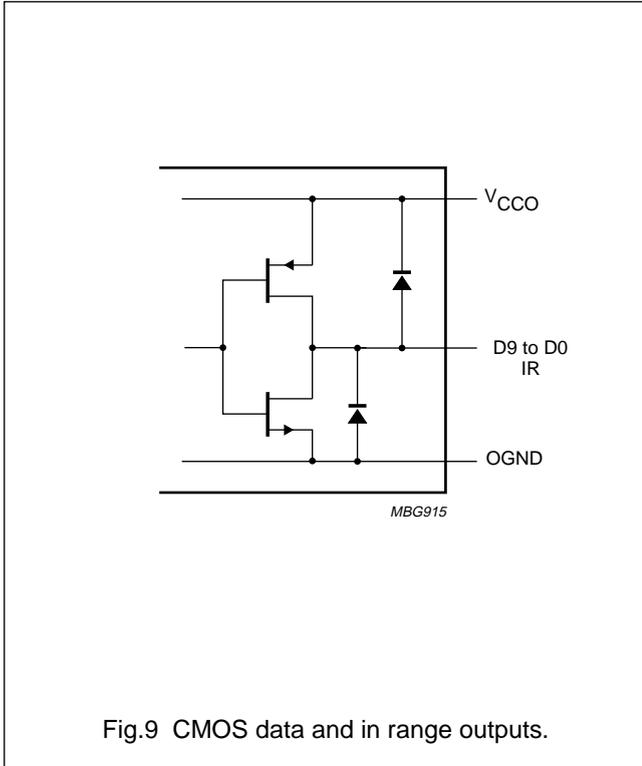
Fig.9 CMOS data and in range outputs.
