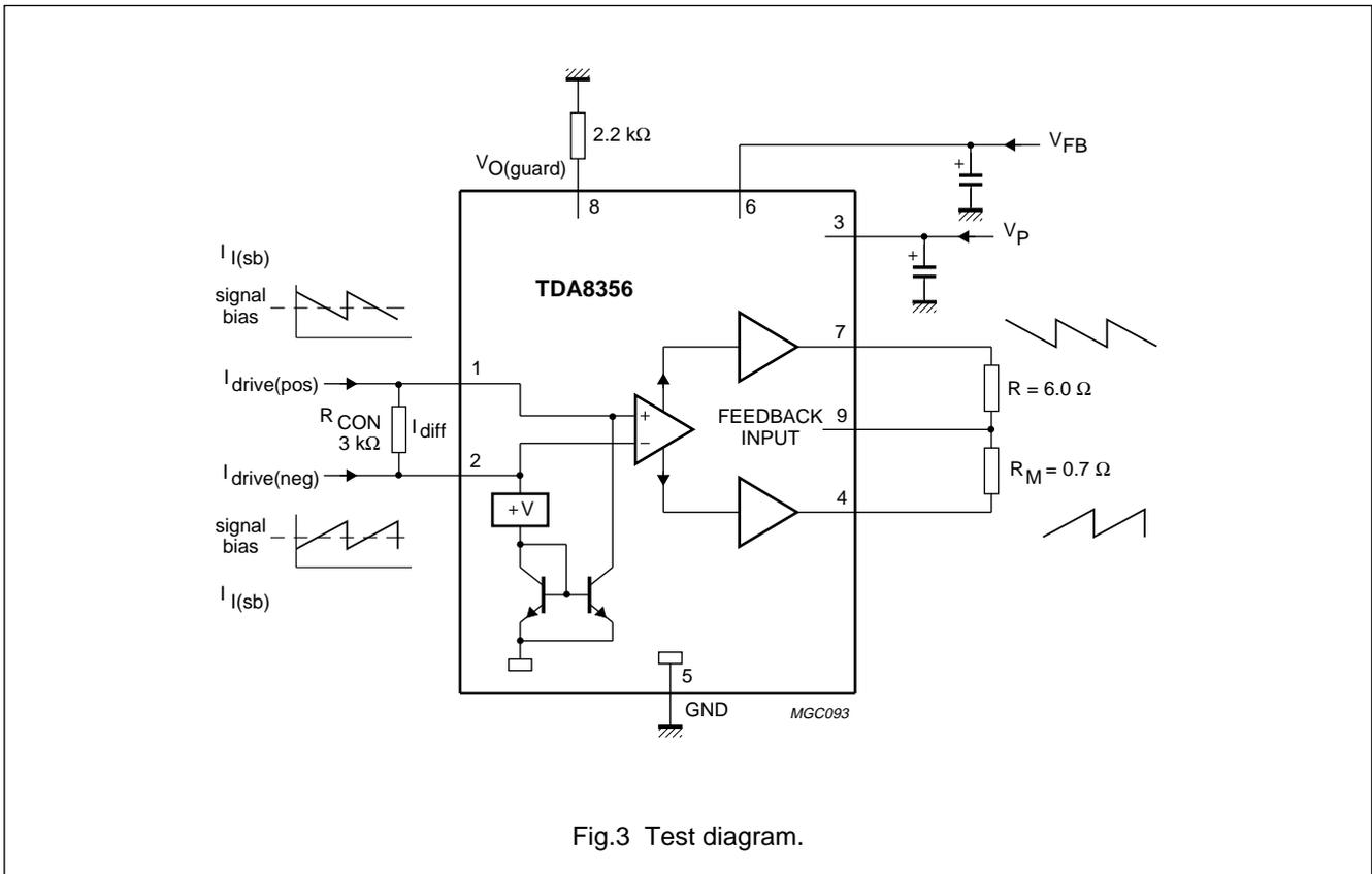
Fig.3 Test diagram.
