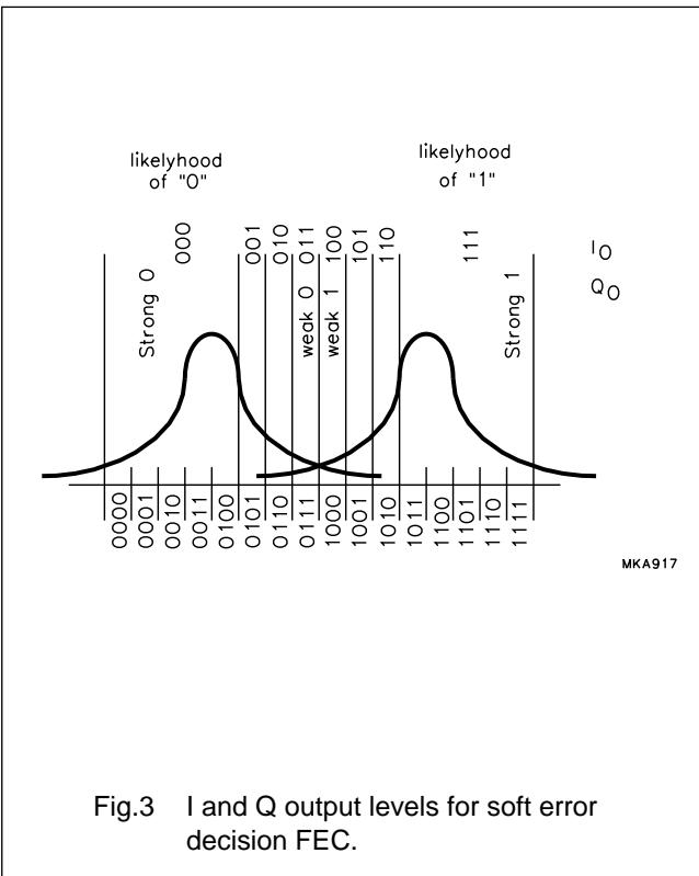
Fig.3 I and Q output levels for soft error decision FEC.
