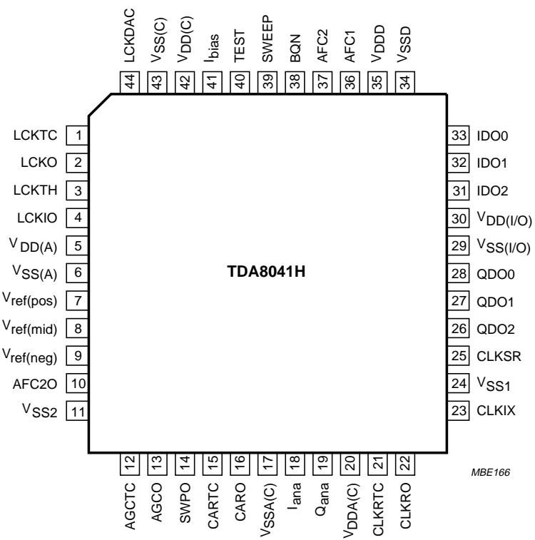
Fig.2 Pin configuration.
