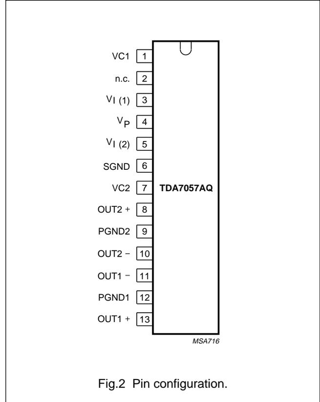
Fig.2 Pin configuration.
