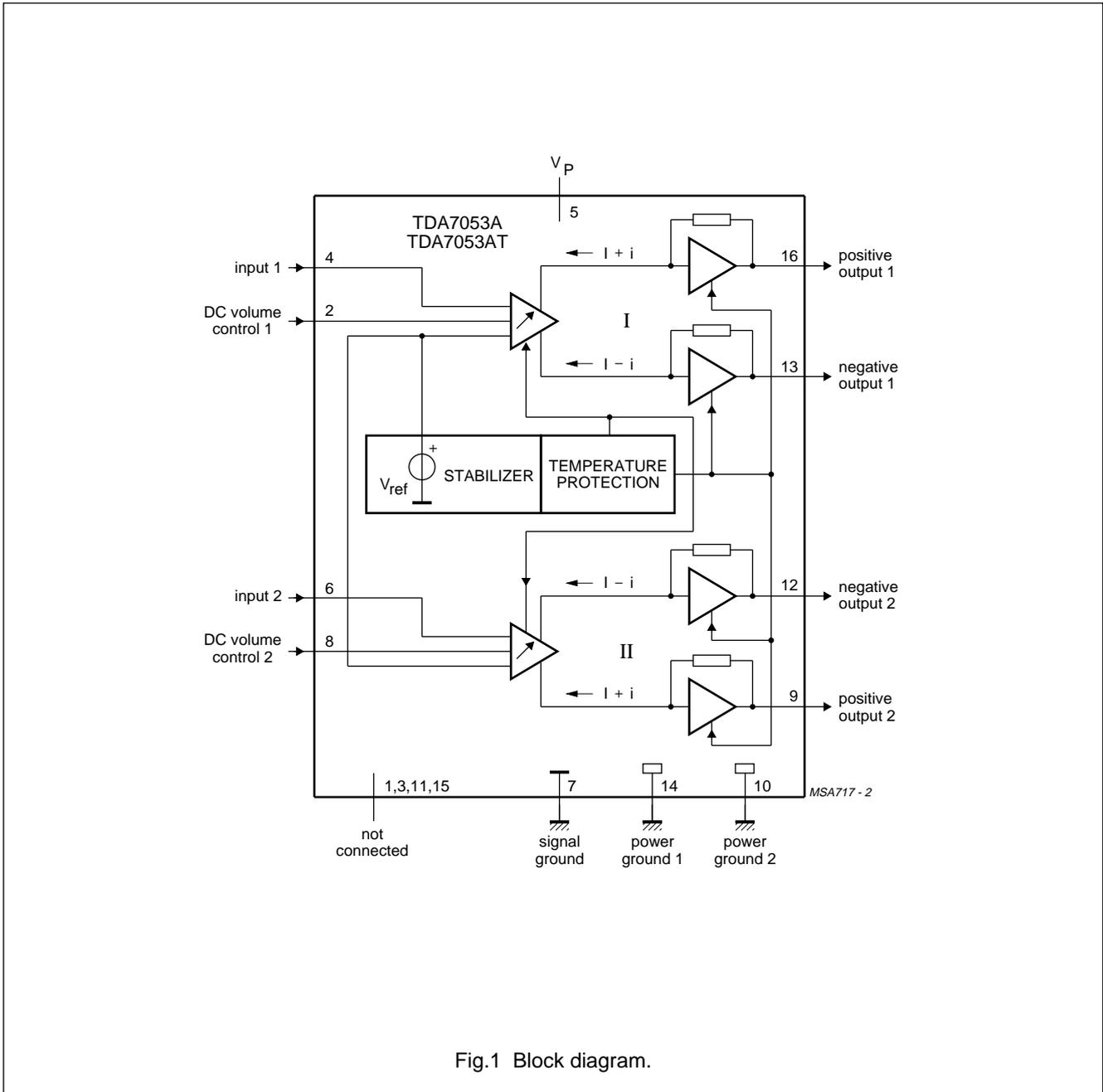
Fig.1 Block diagram.
