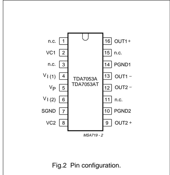
Fig.2 Pin configuration.
