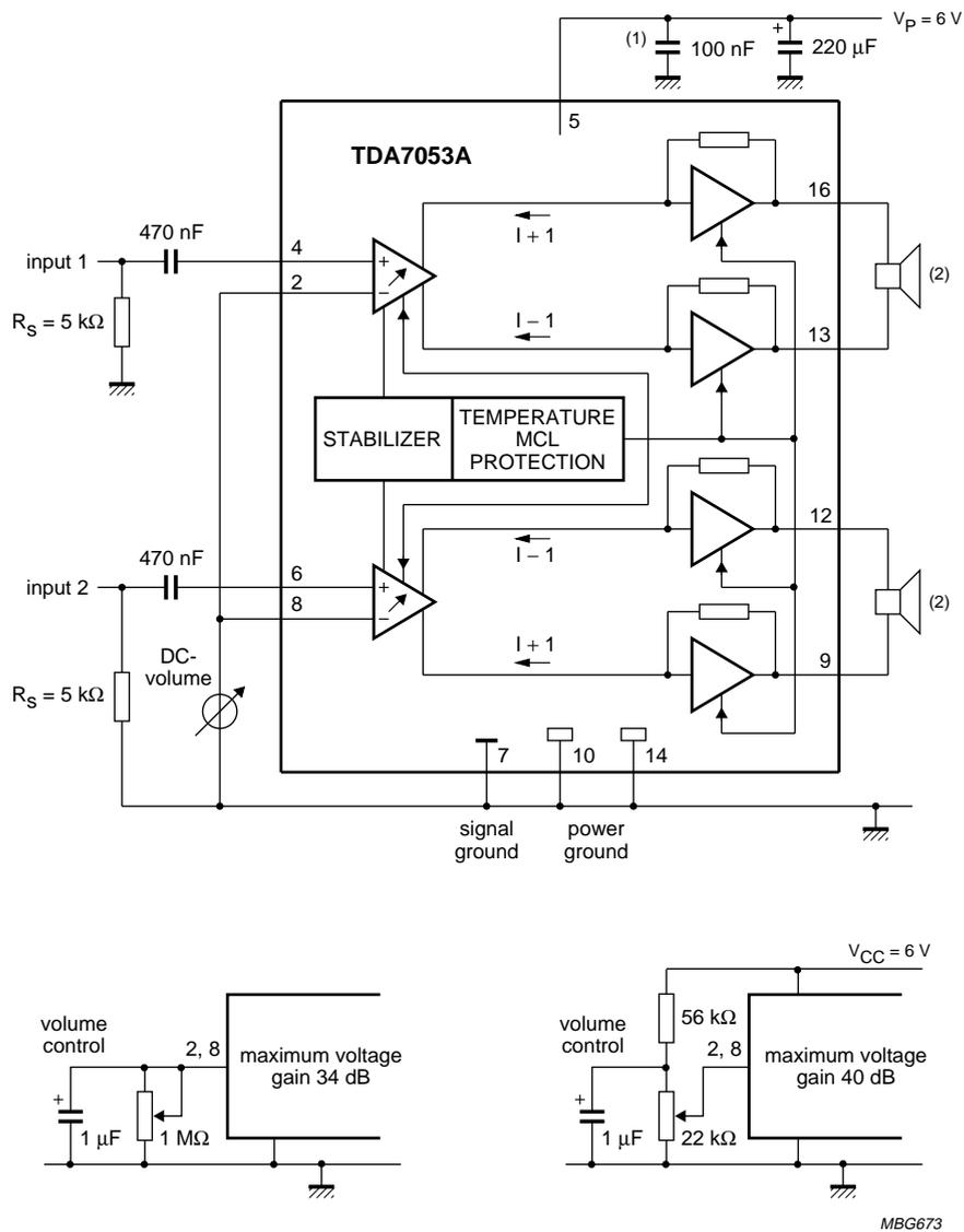
(1) This capacitor can be omitted if the 220 μF electrolytic capacitor is connected close to pin 5.
