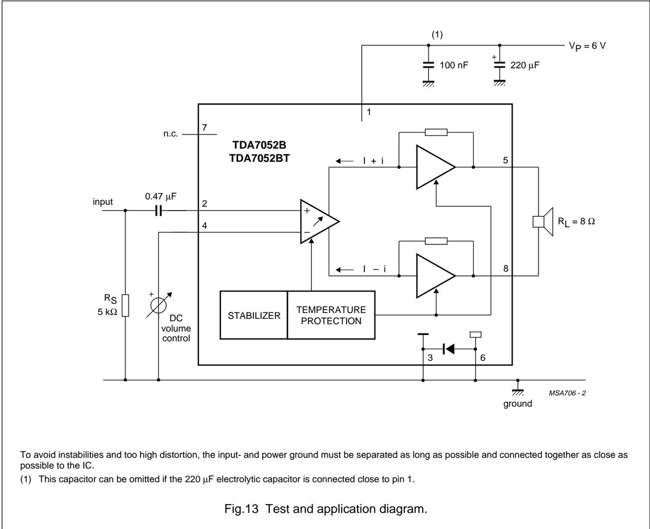
For single-end application the output peak current may not exceed 100 mA; at higher output currents the short circuit protection (MCL) will be activated.
