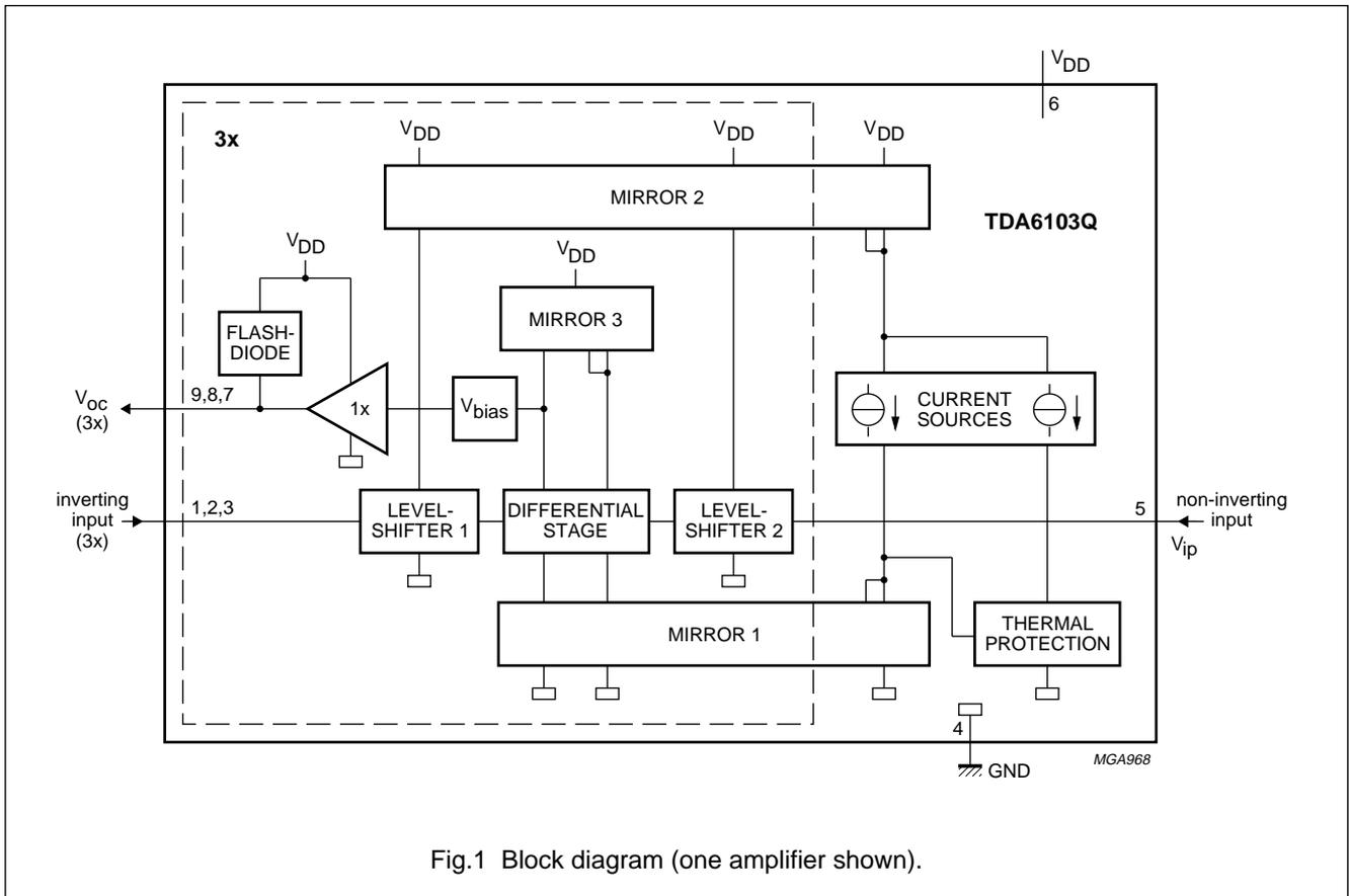
Fig.1 Block diagram (one amplifier shown).
