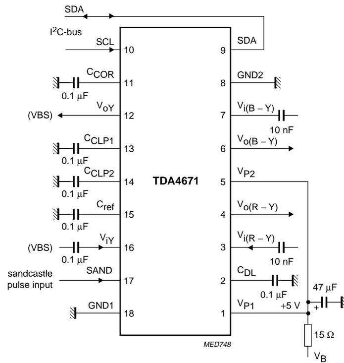
Fig.4 Test and application circuit.
