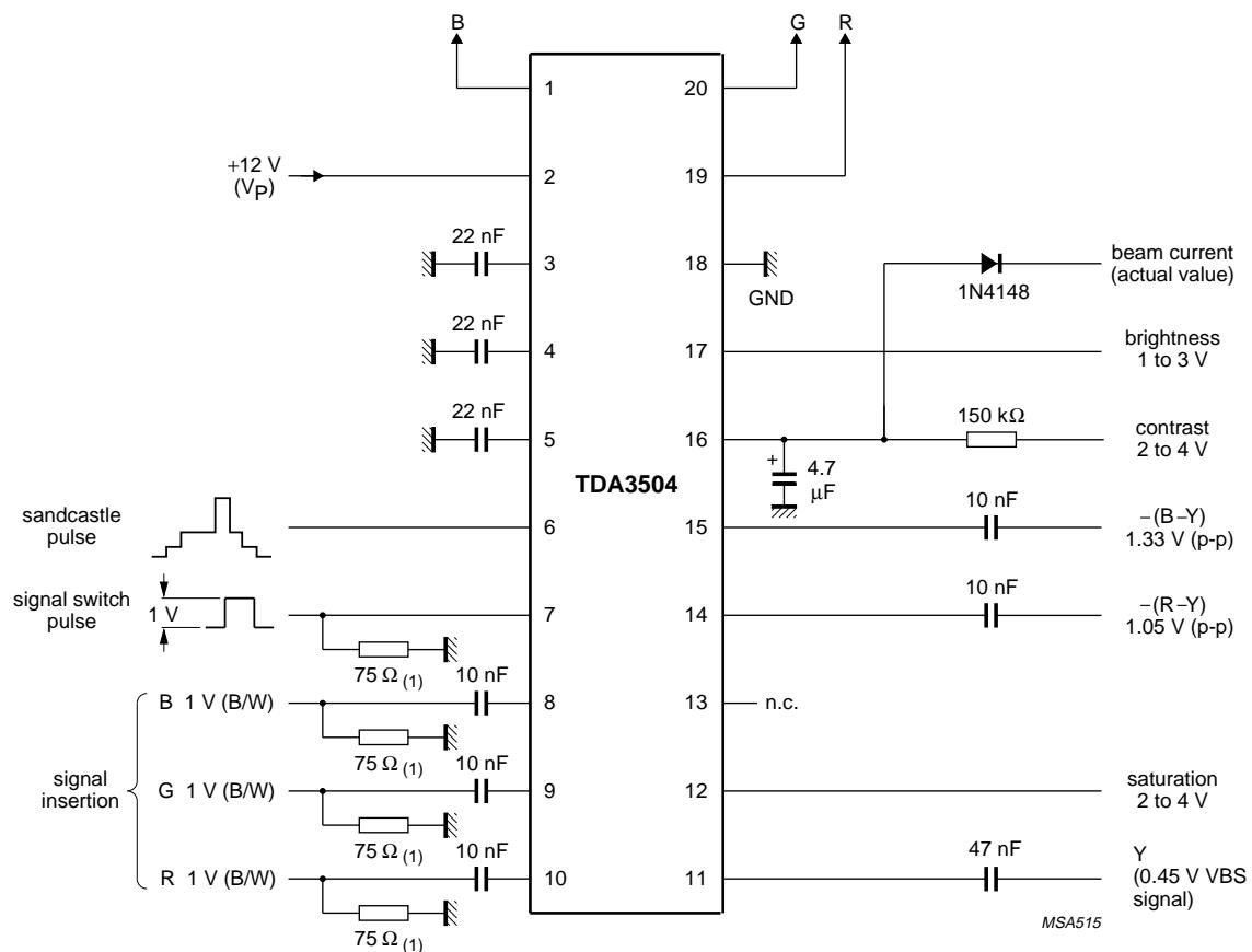
Fig.3 Basic application circuit diagram.
