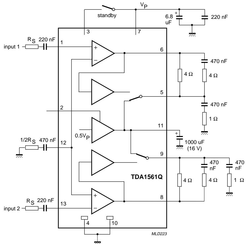
Fig.13 Test diagram.
