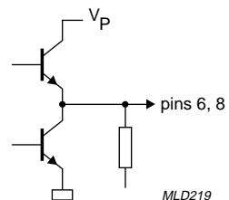
Fig.9 Outputs OUT1 and OUT2.
