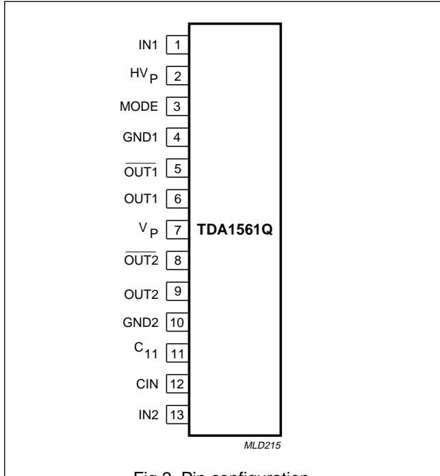
Fig.2 Pin configuration.
