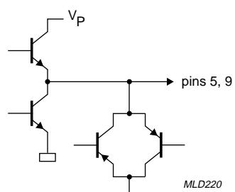
Fig.10 Outputs  $\overline{\text{OUT1}}$  and OUT2.
