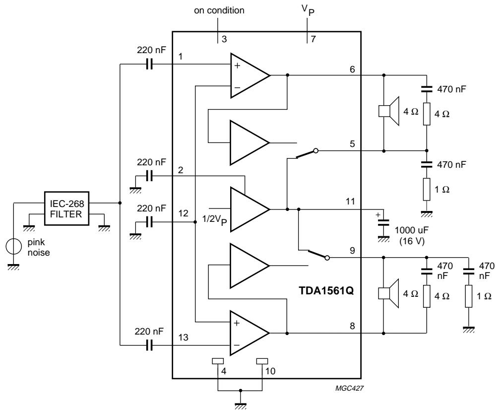
Fig.15 Test and application diagram for dissipation with look alike music signal.
