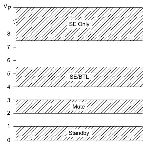
Fig.6 Switching levels of mode select switch.
