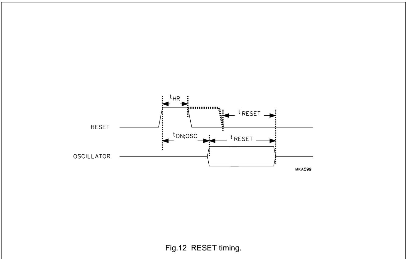
Fig.12 RESET timing.
