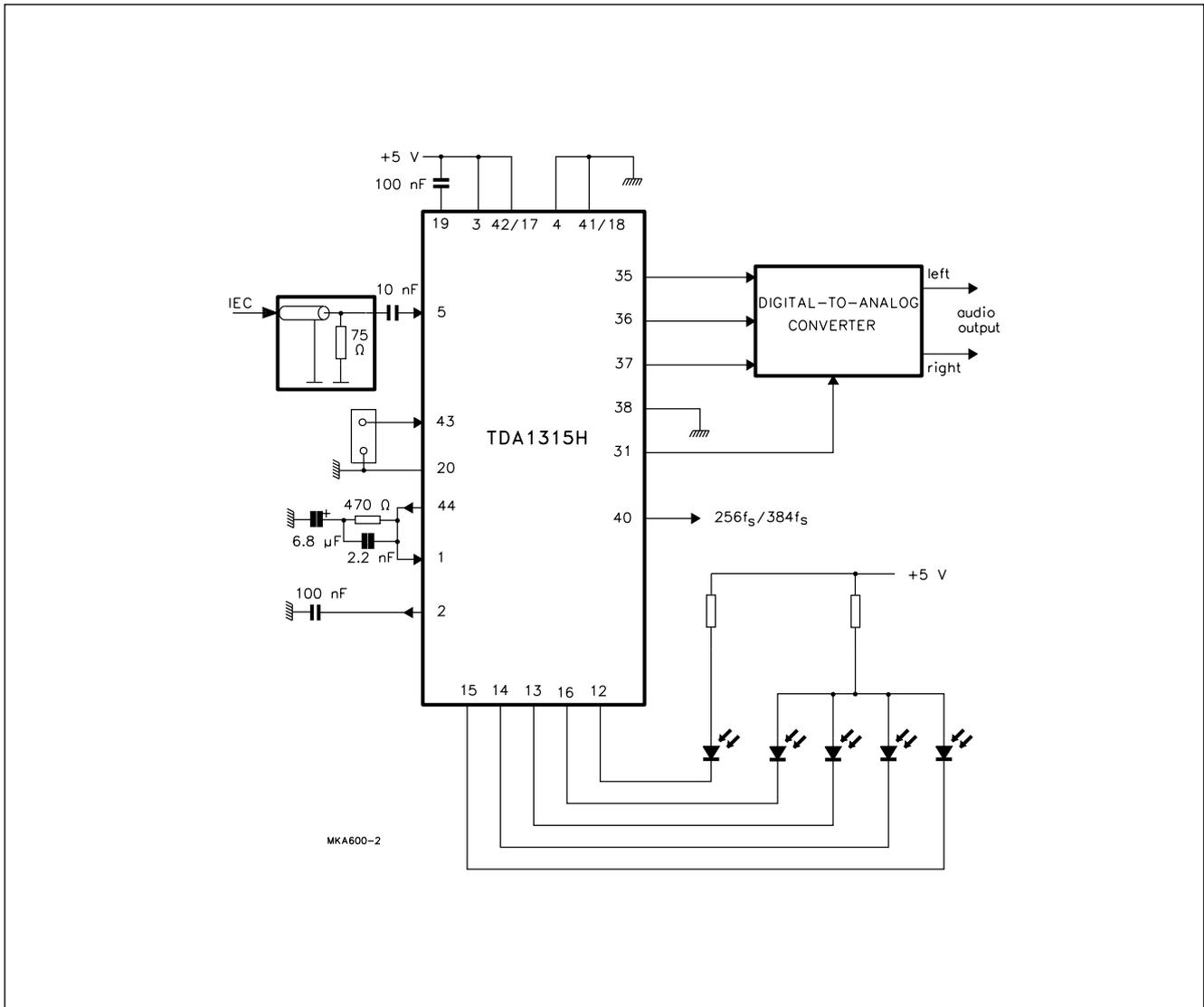
When in a system both IECIN1 and IECIN0 inputs are used, the signal that is applied to the IECIN0 input must be kept away from the IECIN1 input on the printed-circuit board. Steep slopes of the IECIN0 input can be seen by the sensitive adjacent IECIN1 input. An extra capacitance parallel to the 75 Ω resistor, close to the TDA1315H, can help reduce the crosstalk if required. A suitable value is 180 pF.
