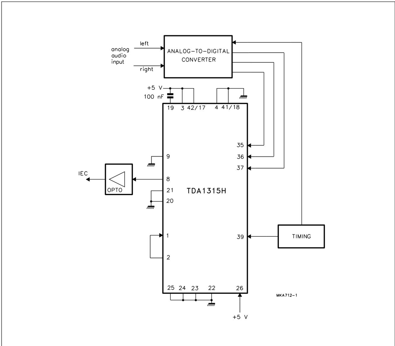
Fig.15 Transmit-mode-only application.
