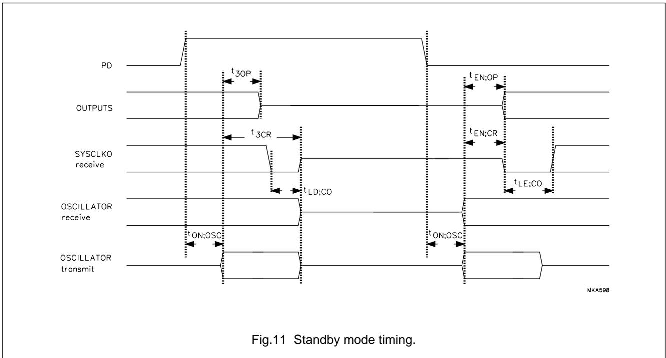
Fig.11 Standby mode timing.
