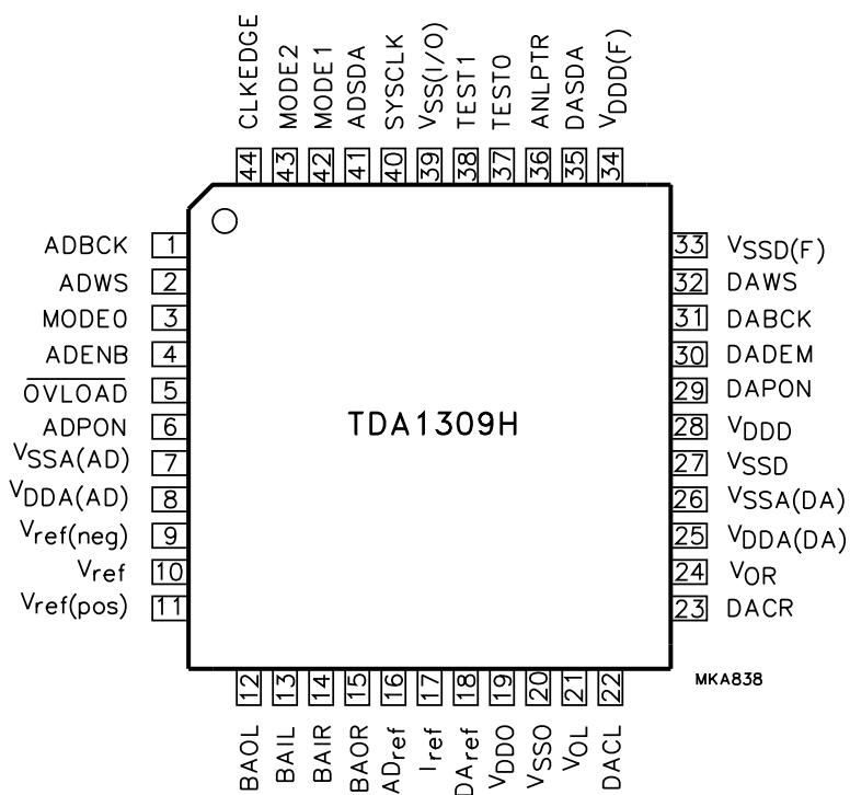
Fig.2 Pin configuration.
