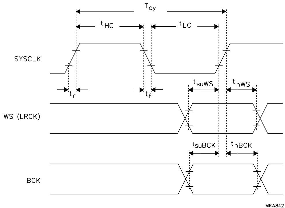
Fig.7 Serial timing of SYSCLK related signals.
