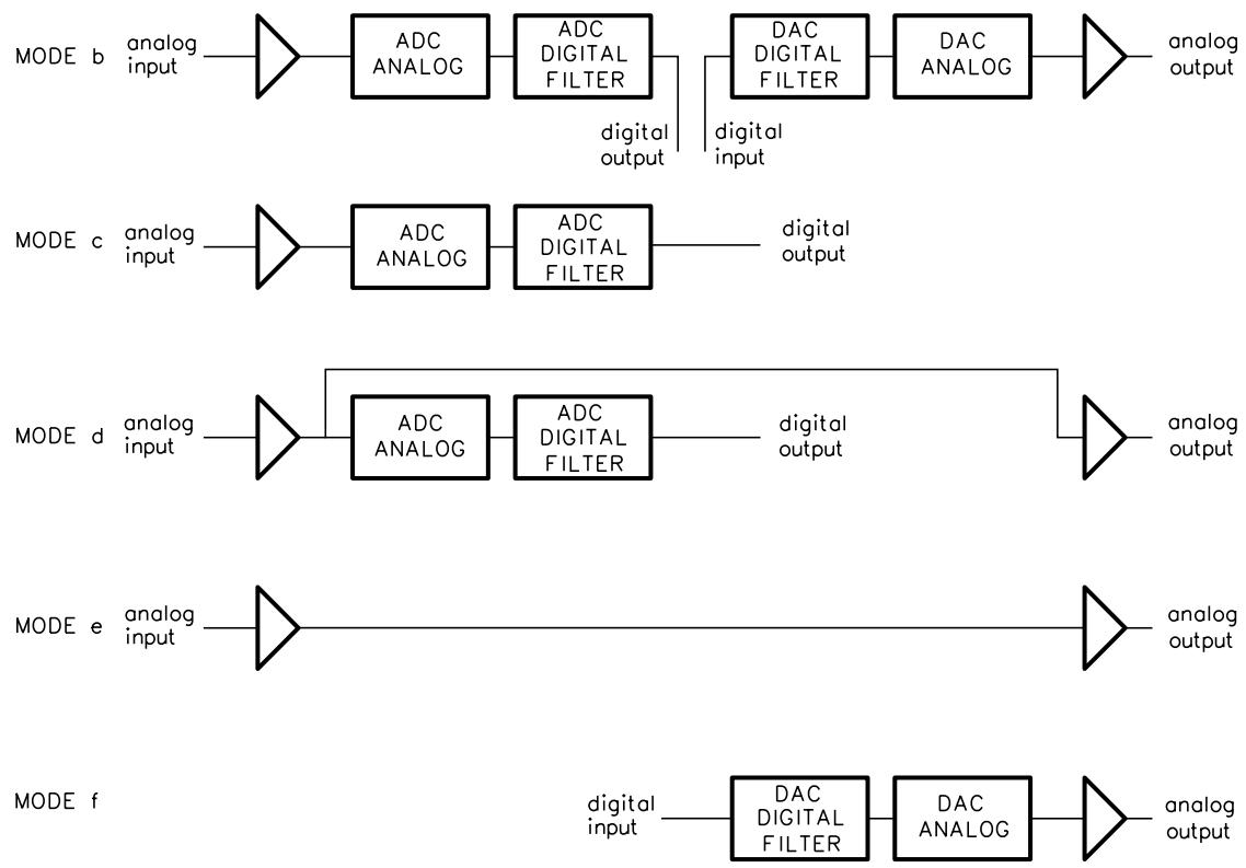
Fig.5 Schematic diagram of operating modes.
