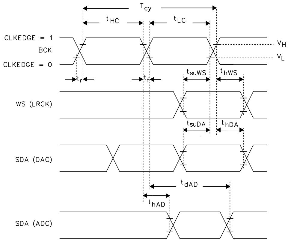
Fig.6 Serial timing of BCK related signals.
