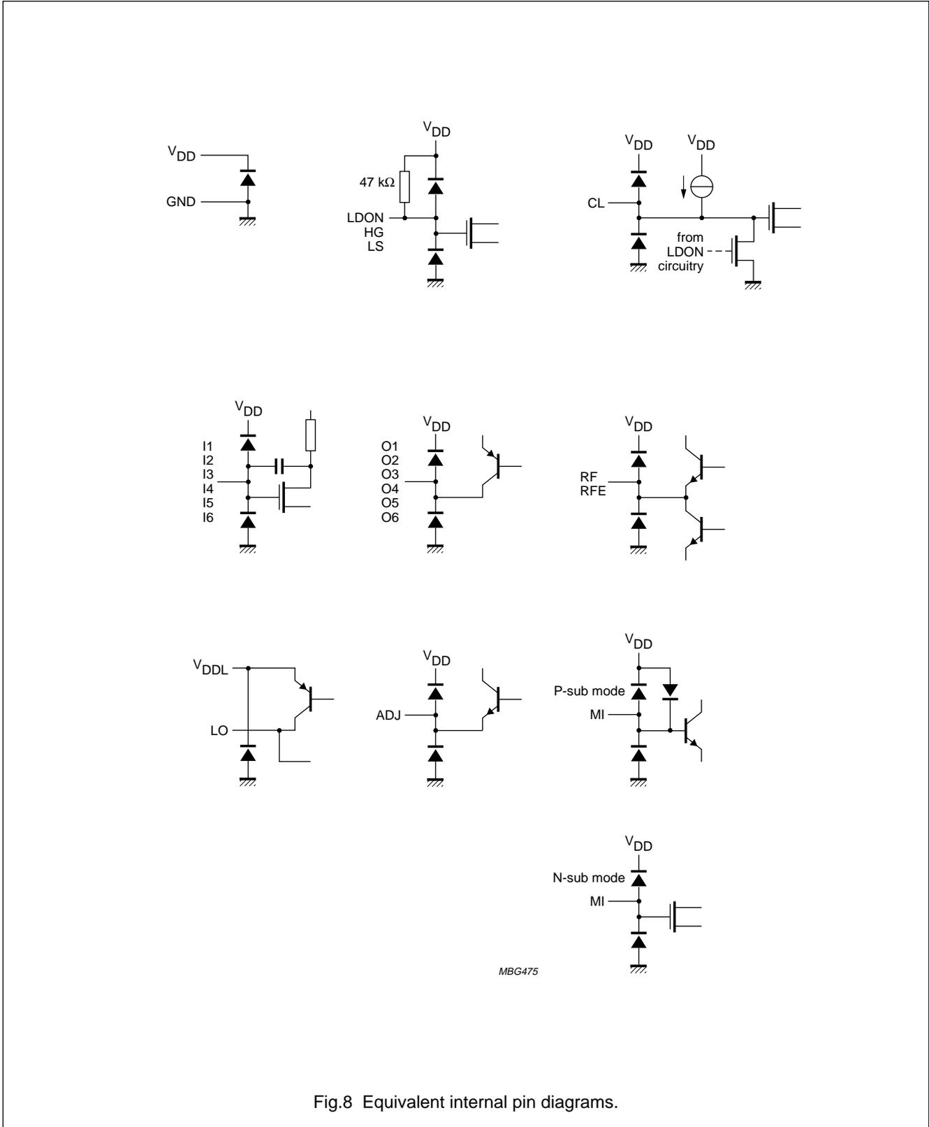
Fig.8 Equivalent internal pin diagrams.
