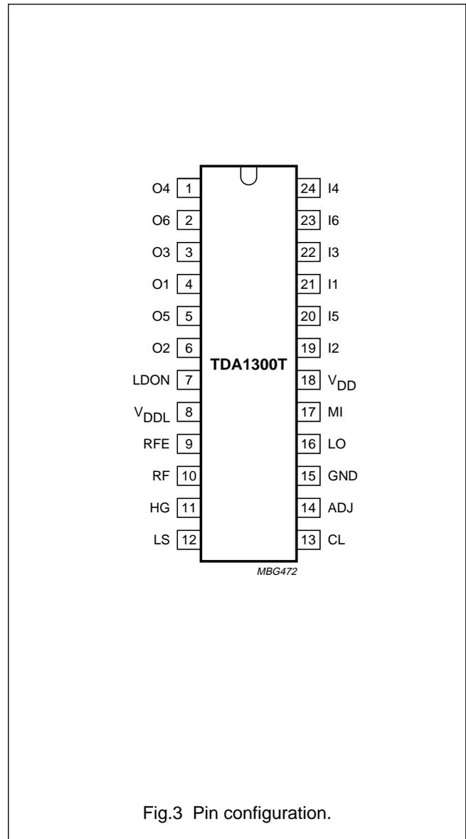
Fig.3 Pin configuration.
