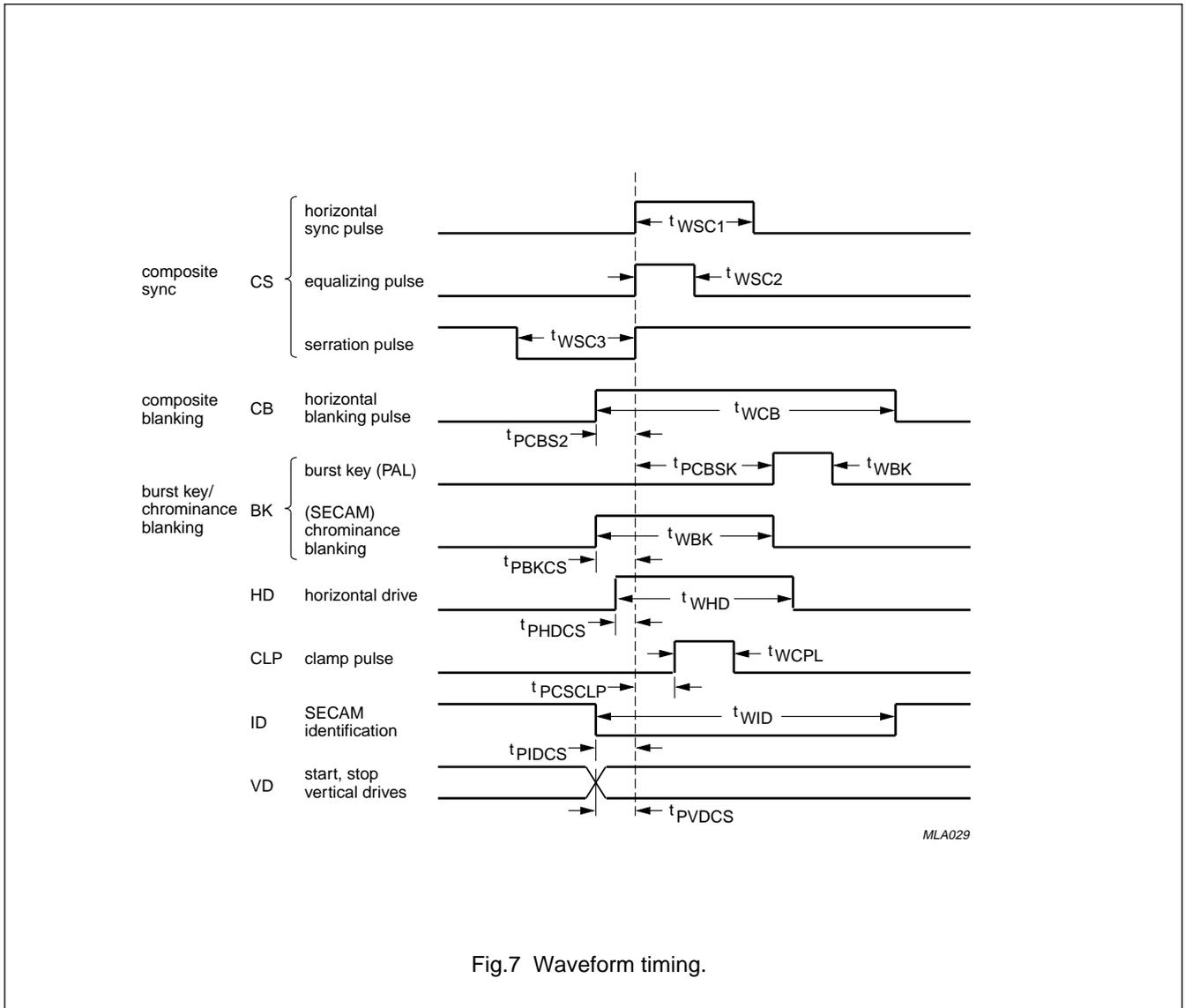
Fig.7 Waveform timing.
