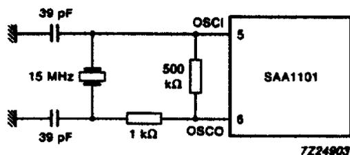
Fig.4 Crystal oscillator circuit.
