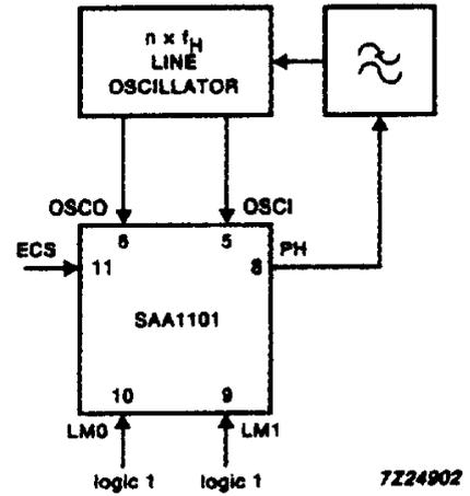
Fig.3 (c) Fast sync lock, internal  $H_{ref}$
