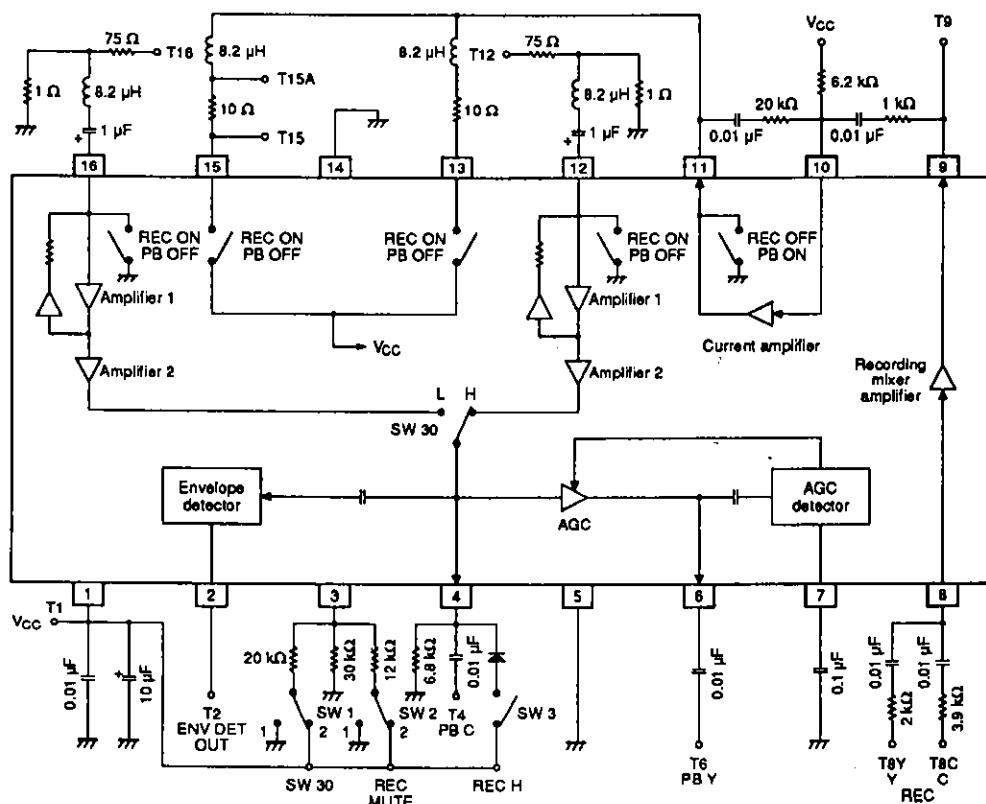
Note that the SW30 switch is in the L position when the voltage on pin 3 is 0 to 1V (muting OFF) or 2 to 3V (muting ON), and in the H position when the voltage on pin 3 is 1 to 2V (muting OFF) or 3 to 4V (muting ON).
