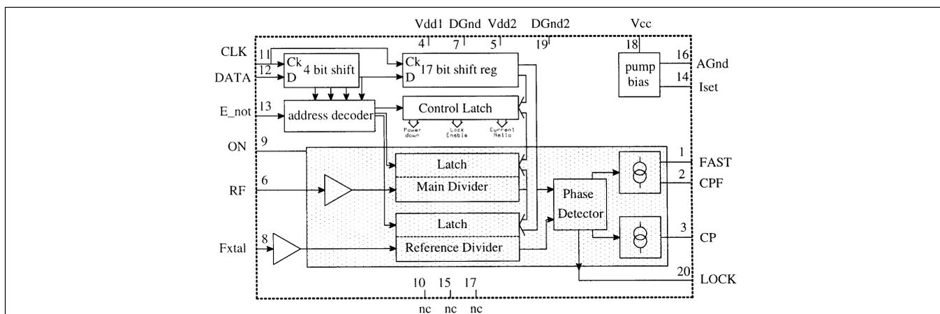
Figure 1–3. UMA1017M and UMA1019M/UMA1019AM Block Diagram
