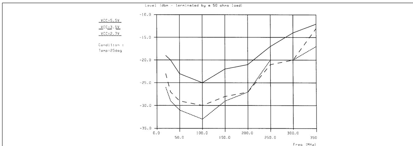
Figure 2-14. Auxiliary Main Divider Input Sensitivity vs Frequency
