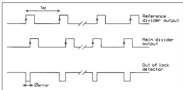
**Figure 2-17. Operating Principal of the Out-of-Lock Detector**
