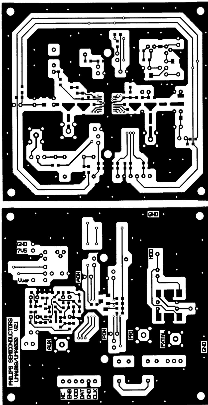
Figure 5-4. Demonstration Board PCB Layout
