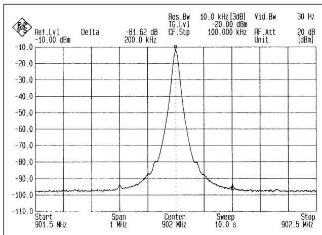
**Figure 4–2. UMA1018M Principal Synthesizer – Comparison Frequency Breakthrough**
