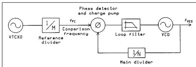
**Figure 3-1. Basic Phase Lock Loop Block Diagram**
