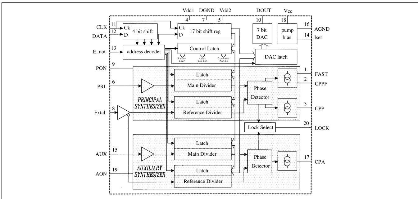
Figure 1-1. UMA1018M Block Diagram
