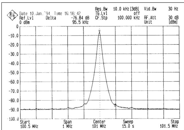
Figure 4-8. UMA1018M Auxiliary Synthesizer – Comparison Frequency Breakthrough
