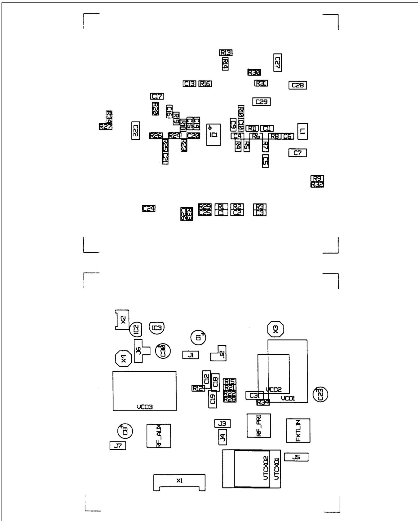
Figure 5-5. Demonstration Board Placement of Components
