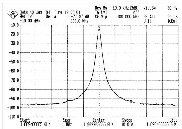
Figure 4-5. UMA1020M Principal Synthesizer – Comparison Frequency Breakthrough
