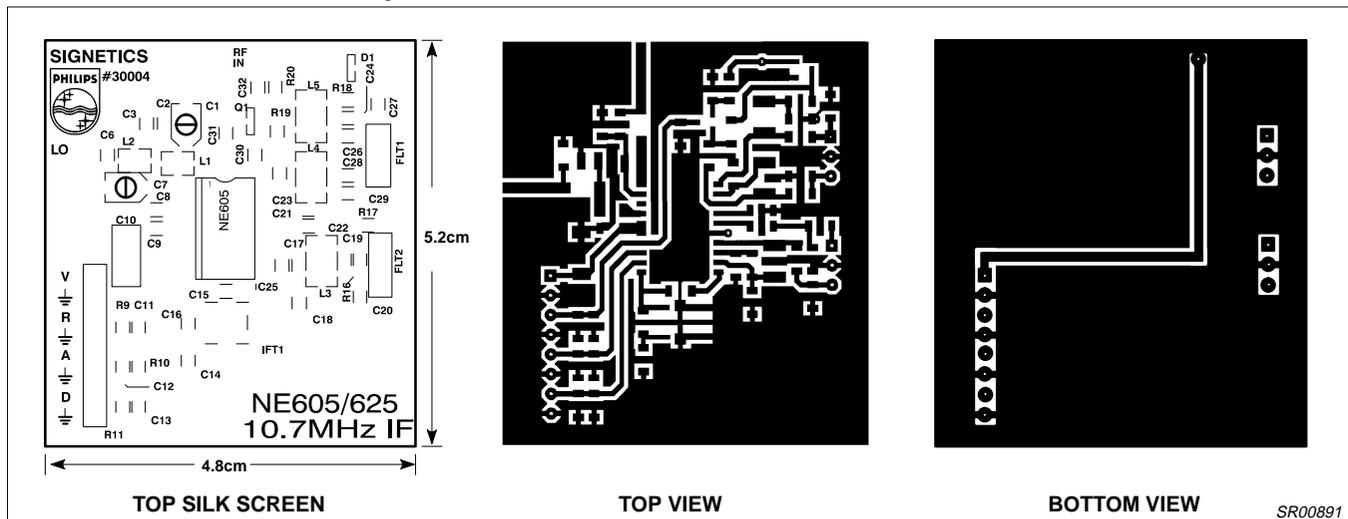
**Figure 3. NE/SA605/625 SO Demo-Board Layouts (Not Actual Size)**
