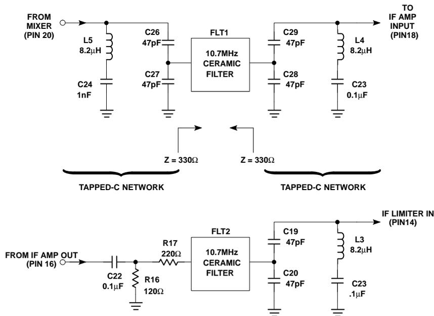
Figure 8. Matching Configuration for FLT1 and FLT2
