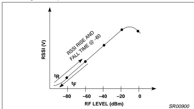
Figure 12. RSSI Curve with Pulsed RF Levels
