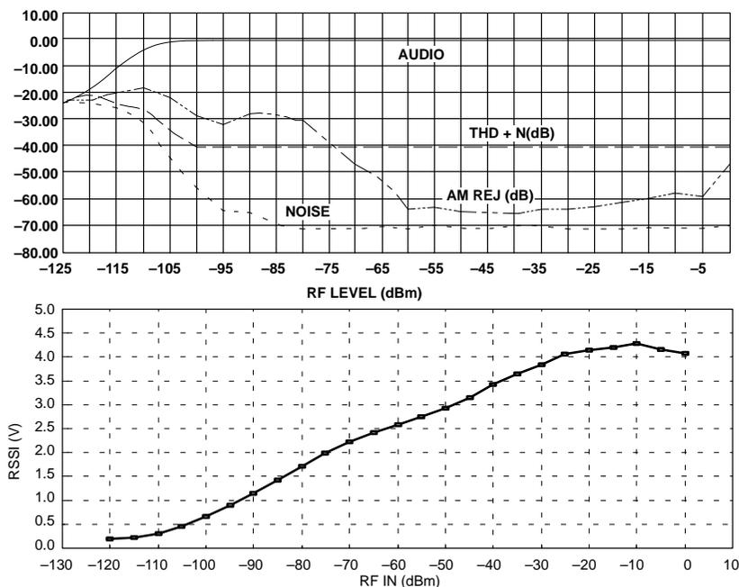
Figure 7. NE/SA605 SO Performance Graphs at 45MHz
