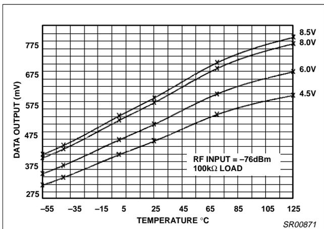
Figure 32. Data Level vs Temperature and Supply Voltage
