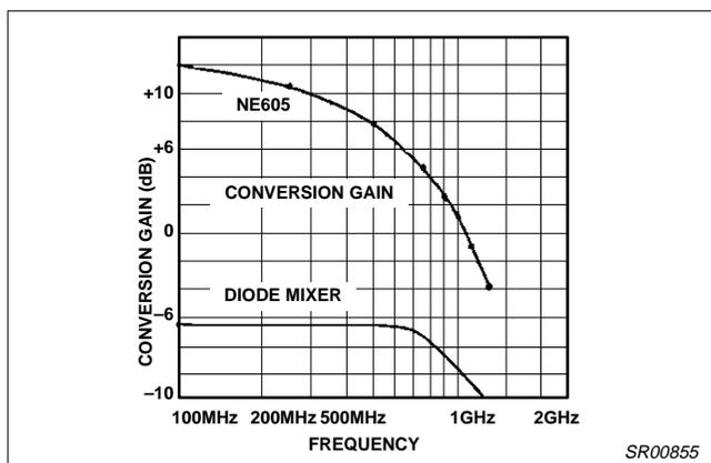
Figure 16. NE605 Conversion Gain vs. Diode Mixer
