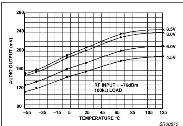
Figure 31. Audio Level vs Temperature and Supply Voltage
