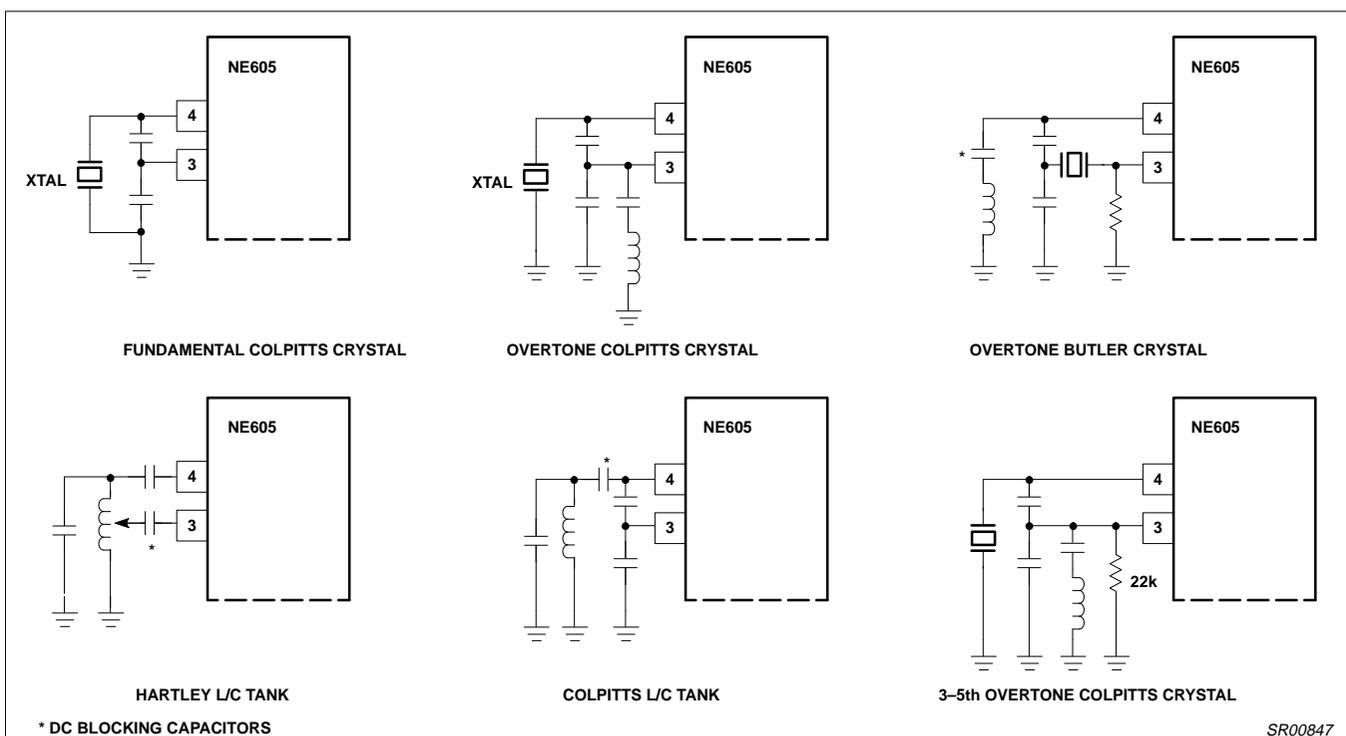
**Figure 8. Oscillator Configurations**
