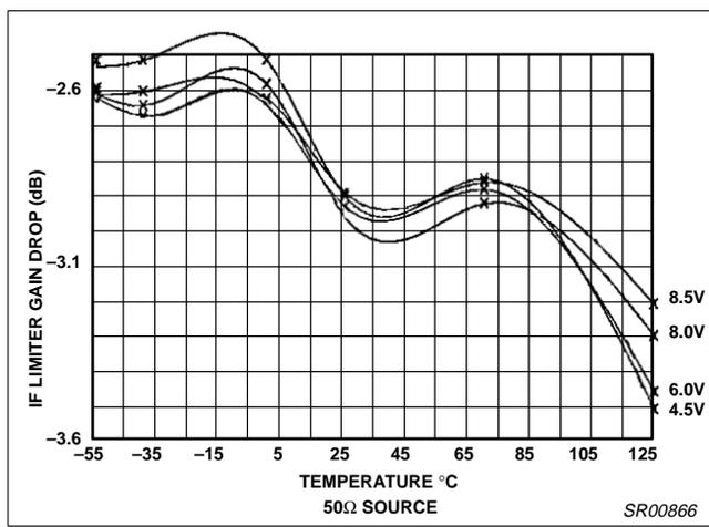
Figure 27. IF Limiter Drop, 20MHz Response
