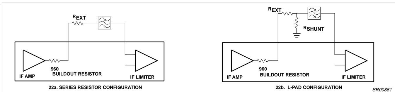
Figure 22. Implementing the 12dB Insertion Loss
