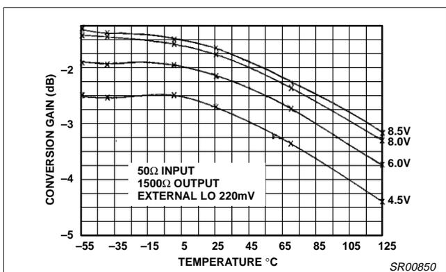
Figure 11. 50Ω Conversion Gain
