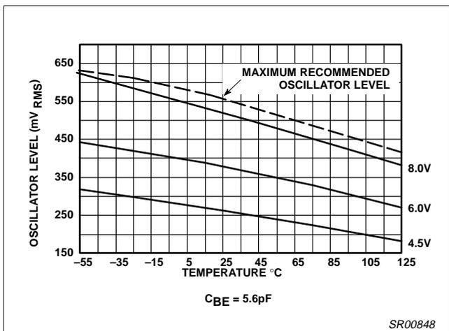
Figure 9. NE605 Application Oscillator Level
