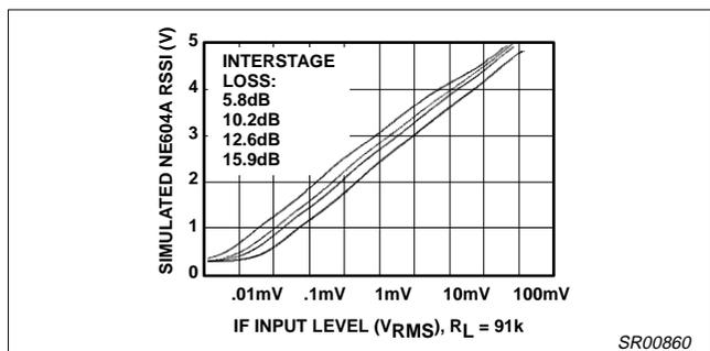
Figure 21. NE604A's RSSI Curve at Different Interstage Losses
