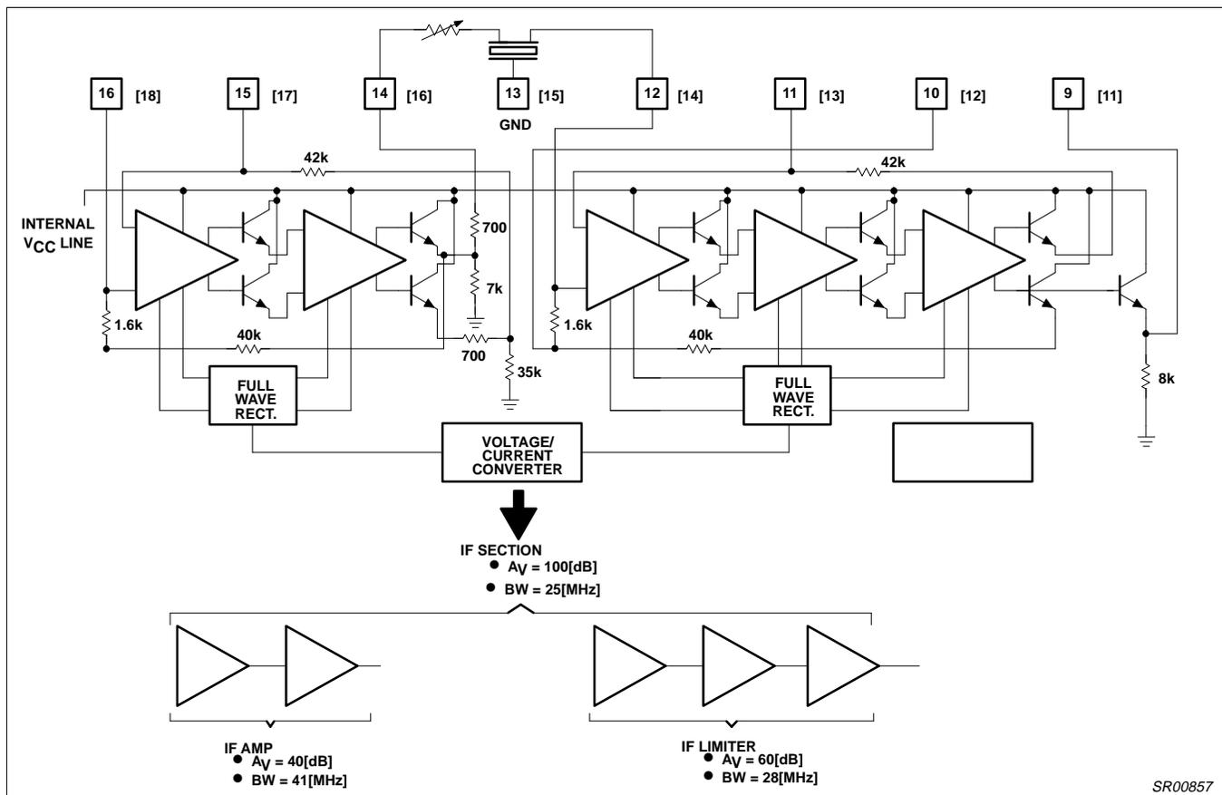
Figure 18. IF Section of NE604A [NE605]
