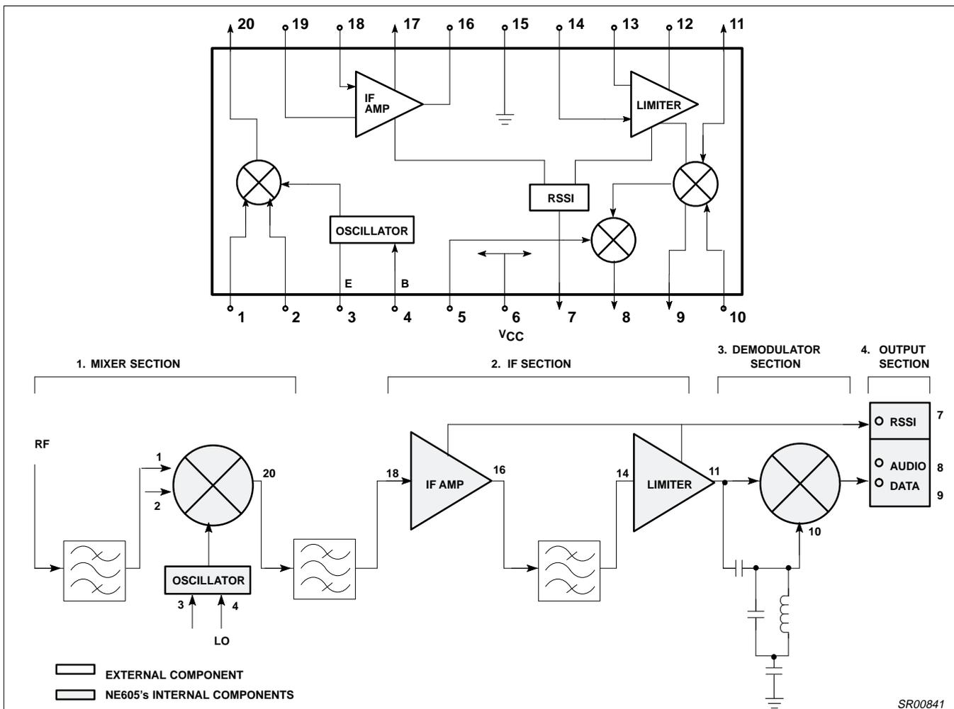
Figure 2. NE605 Broken Down into Four Areas
