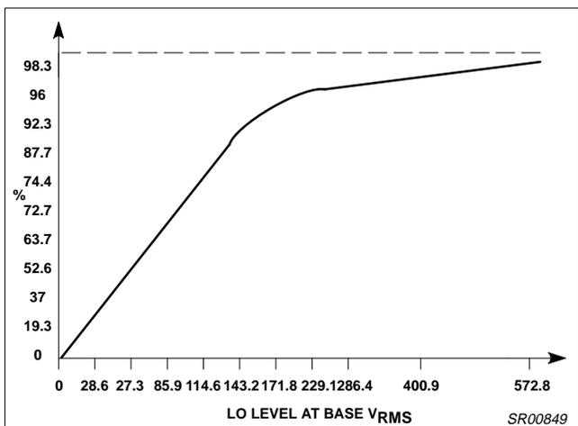
Figure 10. Mixer Efficiency vs. Normalized LO Level
